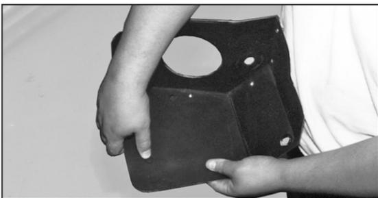
13. Insert the grommets provided, into the holes onto the bottom side of the heat shield.
