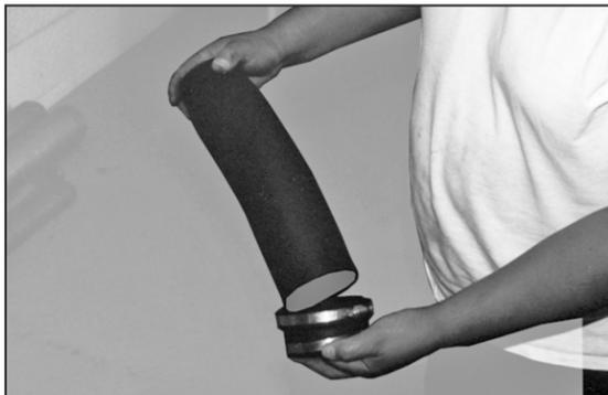
20. Install the hose clamps on the tube adapter and install this assembly onto the intake tube.
