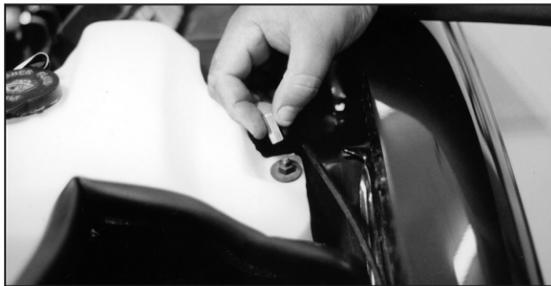
17. Thread the provided coupling nut onto the stud that protrudes through the windshield washer reservoir. Tighten down securely.
