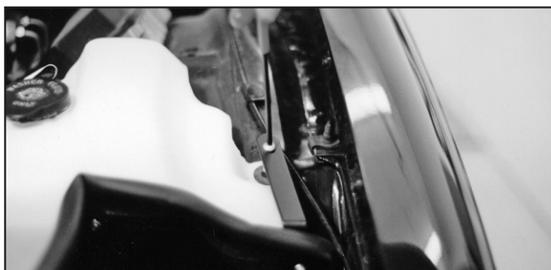
19. Attach the bracket to the coupling nut with the provided bolt. Tighten down securely.
