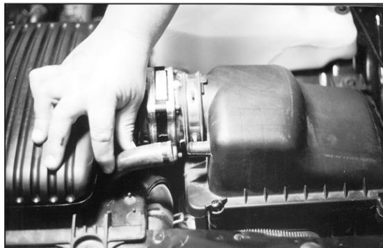
5. Detach the air injection hose from the airbox.
