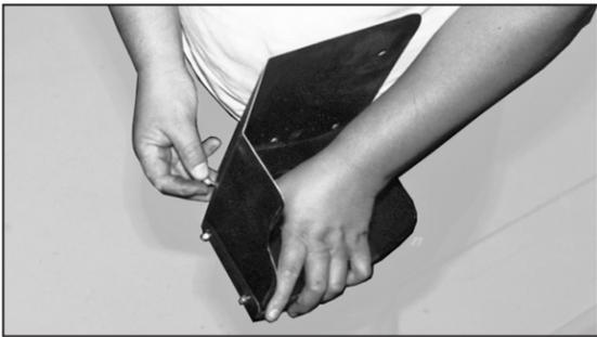
11. Assemble the heat shield by using nylock nuts and allen head bolts provided.
