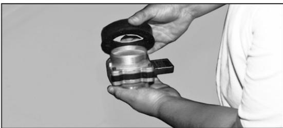
14. Install the filter adapter onto the mass air sensor. The notch in the adapter aligns with the tab on the mass air sensor.
