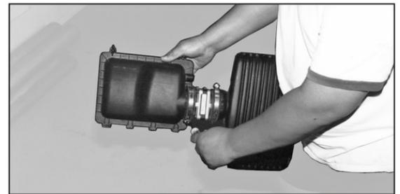
7. Remove the mass air sensor from upper airbox sound chamber housing.
