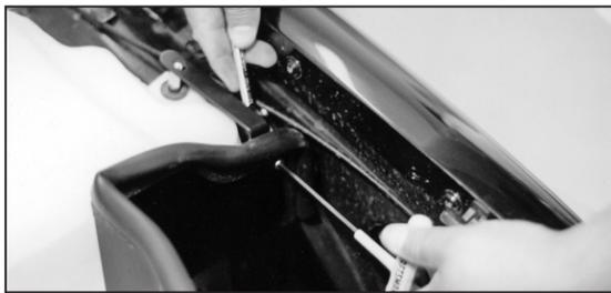
18. Attach the bracket to the heat shield with the provided hardware. As shown in the parts list above. Tighten down securely.
