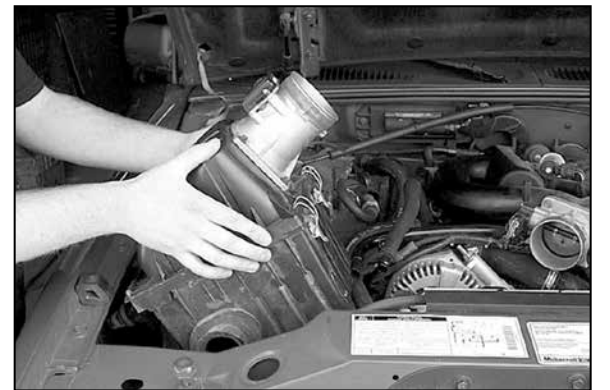
6. Using a screw driver, pry the air cleaner assembly upwards to release the air cleaner from the factory grommets, then remove the air cleaner assembly.
