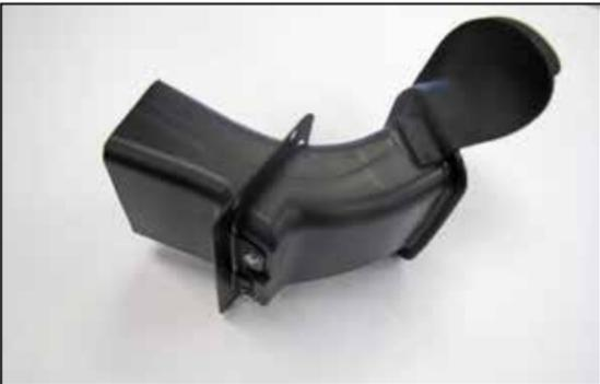
10. Install the provided fresh air scoop mounting bracket onto the fresh air scoop and secure with the provided hardware.
