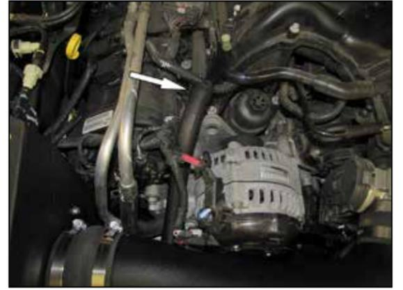
17. Install the provided crank case vent line onto the fitting installed into the intake tube and onto the factory hardline.
