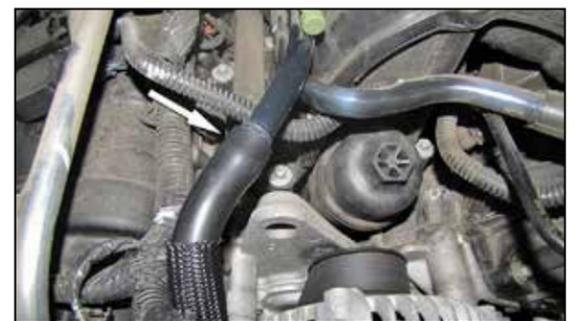
5. Disconnect the crank case vent flex line from the hardline at the connection shown.
