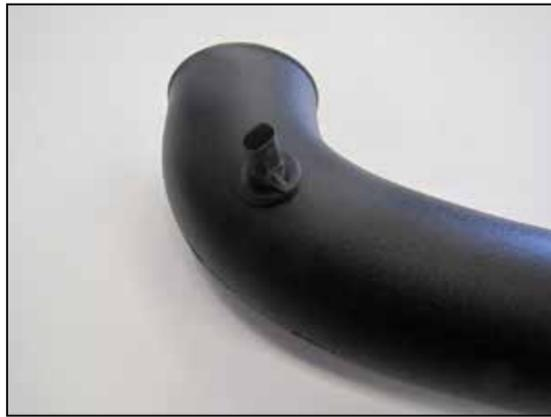
14. Remove the inlet air temperature sensor from the factory intake tube. Using the provided grommet install the inlet air temperature sensor into the K&N® intake tube.
