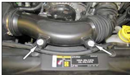
3. Remove the two bolts that secure the factory intake tube to the fan shroud.
