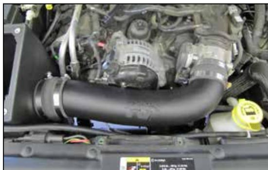
16. Install the provided hump coupler (08699) onto the K&N® intake tube and then install the assembly into the vehicle. Adjust the tube for best fit and then secure with the provided hose clamps. Reconnect the inlet air temperature sensor electrical connection.
