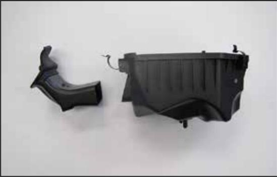
9. Using a 1/8" drill, drill out the two rivets that secure the factory fresh air duct to the factory air filter housing and then remove the duct from the housing as shown.
