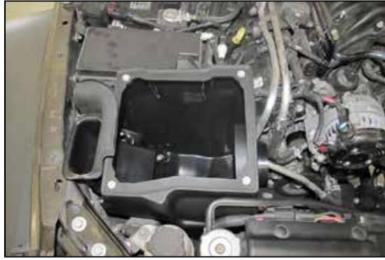
12. Install the K&N® air filter housing into the vehicle so the mounting studs insert into the factory mounting brackets.
