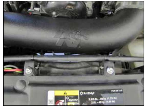
19. Install the "L" brackets onto the fan shroud using the provided hardware and then secure the coolant hose with the tie wraps.
