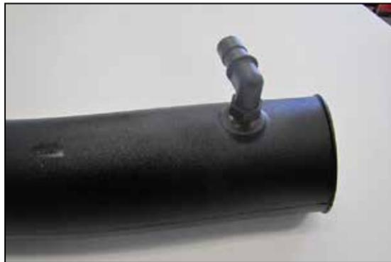
15. Install the provided 90° fitting into the K&N® intake tube as shown.
