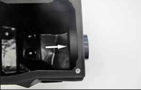
8. Install the provided filter adapter into the housing and secure with the provided hardware.
