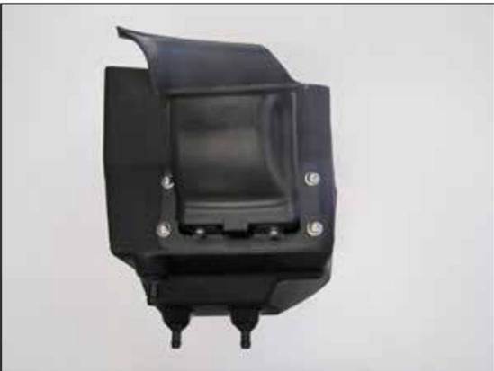
11. Install the fresh air intake assembly into the K&N® air filter housing and secure with the provided hardware.
