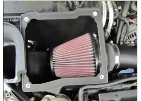
20. Install the K&N® air filter onto the adapter and secure with the provided hose clamp.
