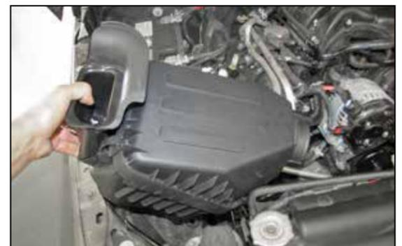
6. Remove the factory air filter housing from the vehicle.
