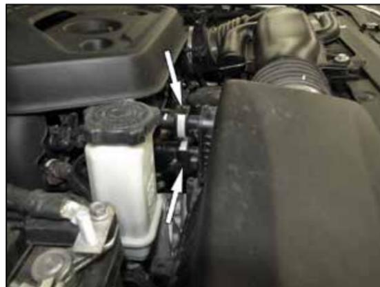
3. Depress the locking tab and disconnect the two vent lines from the air filter housing.
