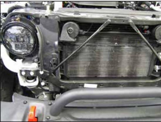
9. Reinstall the core support diagonal brace using the factory hardware.
