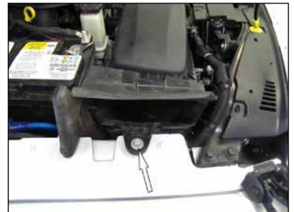
5. Remove the bolt that secures the fresh air duct to the fender. Remove the complete intake system from the vehicle.
