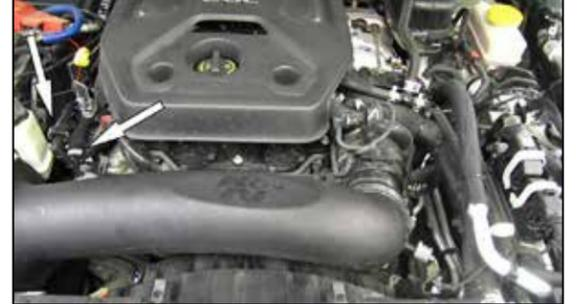
18. Connect the CCV lines to the ejection fitting installed into the intake tube.
