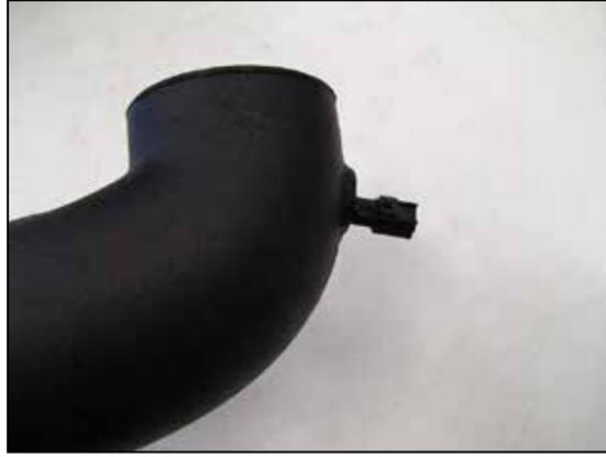
13. Remove the inlet air temperature sensor from the factory intake tube. Remove the O-ring from the sensor and then install the sensor into the K&N® intake tube using the provided grommet.
