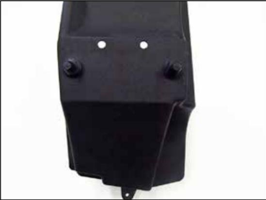
11. Install the provided mounting post onto the K&N® air filter housing using the provided hardware.
