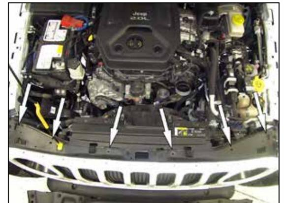
6. Remove the six retaining clips that secure the grill assembly to the core support. Remove the grill assembly.
