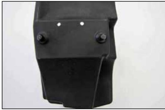
11. Install two airbox mounts onto the K&N airbox with provided hardware.
