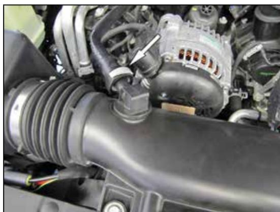
3. Disconnect the crank case vent line.
