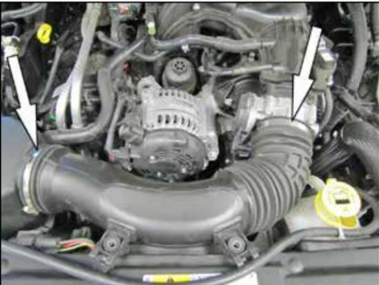
4. Loosen the hose clamps securing the intake tube. Disconnect the inlet air temperature sensor and then remove the intake tube from the vehicle. **NOTE: The inlet air temperature sensor is located under the intake tube and is very fragile, use caution while handling the sensor.**
