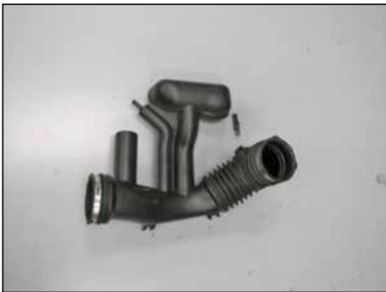
35. Remove the inlet air temperature sensor from the factory intake tube.
