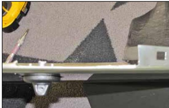
53. Using a cut-off wheel or similar tool, cut along the lines marked with the template and remove that section of the fender. Be sure to remove any remaining burrs with a file or deburring tool.
