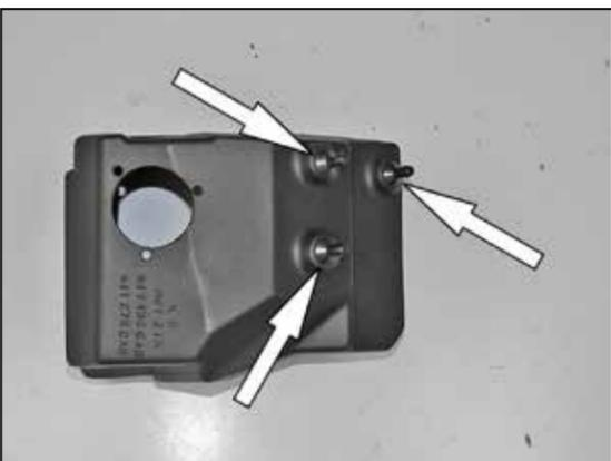
21. Using the provided hardware, attach the three provided mounting studs to the K&N® air filter housing.
