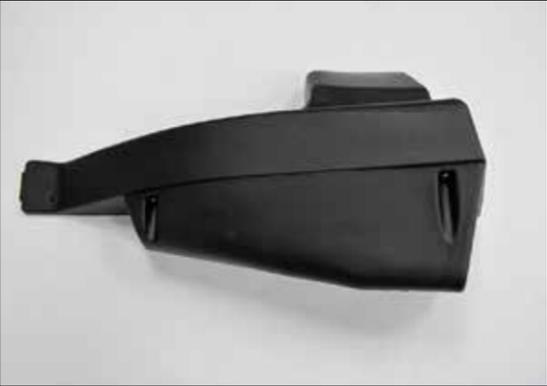
5. Assemble the right side K&N® prefilter/scoop by placing the prefilter onto the housing and then installing the scoop onto the housings and secure with the provided hardware.
