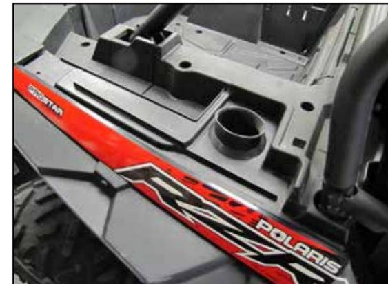
3. Remove the factory prefilters from the vehicle.
