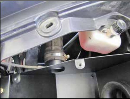
22. Connect the fresh air intake hose to the air filter box and secure with the factory hose clamp.
