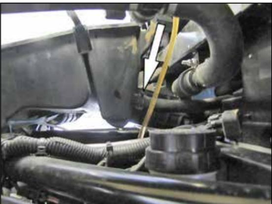
10. Reach through the driver's side wheel opening and locate the crank case vent hose attached to the rear of the air filter housing. Release the spring clamp and disconnect the crank case vent hose from the air filter housing.
