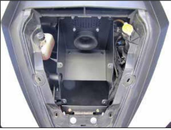
21. Set the air box into position and secure it to the K&N® bracket with the hardware provided. Secure the front of the box with the factory air filter housing bolts removed earlier.
