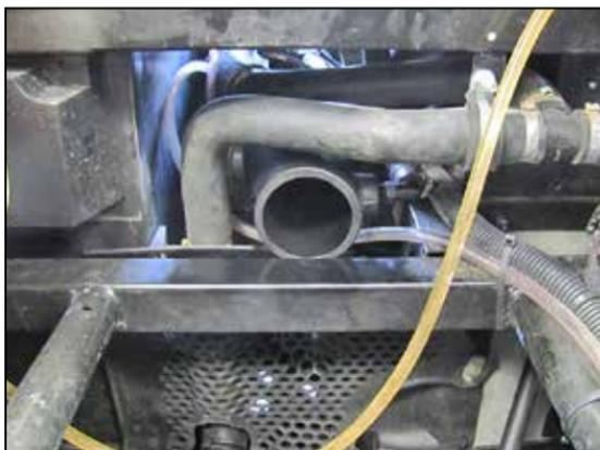
15. Install the K&N® intake tube into the coupler hose at the throttle body, the vent fitting should be on the driver's side of the vehicle and on the front of the tube. Connect the crank case vent hose to the fitting installed into the K&N® intake tube and secure with the factory spring clamp.
