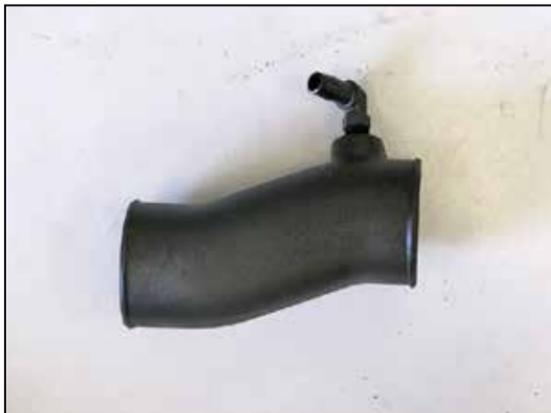
14. Install the provided 90° fitting into the K&N® intake tube.
