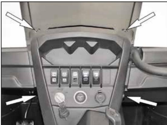
2. Remove the two bolts and two plastic clips securing the center dash, then remove the center dash and set aside to gain access to the intake system.
