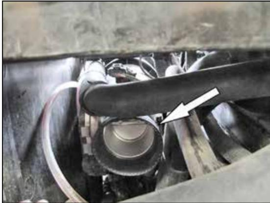
13. Install the provided coupler (08440) onto the throttle body and secure with the provided hose clamp.
