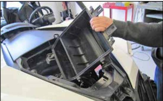
11. Have an assistant lift up the front of the body work, then pull the air filter housing forward and disconnect the intake tube from the throttle body. Rotate the air filter housing counter clockwise 90° and guide it out through the opening in the body work to remove it from the vehicle.
