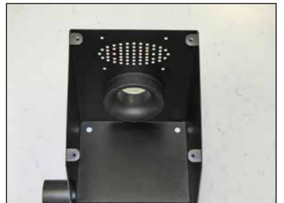
19. Install the radius adapter into the air filter box and secure with the provided hardware.
