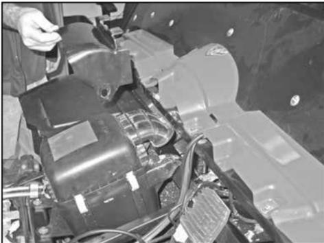
13. Remove the deflector shield as shown.
