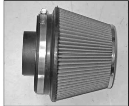
22. Install the provided filter adapter into the K&N® air filter and secure with the provided hose clamp.
