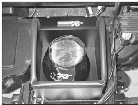
26. Install the K&N® air filter assembly onto the intake tube and secure with provided hose clamp.
