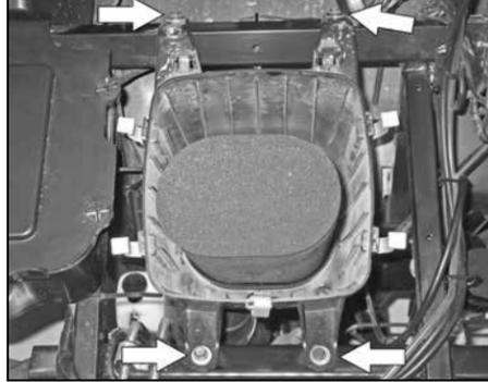
15. Remove the four air box mounting bolts shown.
