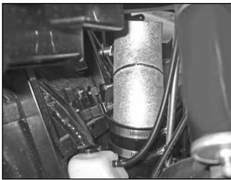
25. Install the K&N® intake tube into the silicone hose and align with the tube mounting bracket installed onto the heat shield, then secure the intake tube with the hose clamp and hardware provided.
