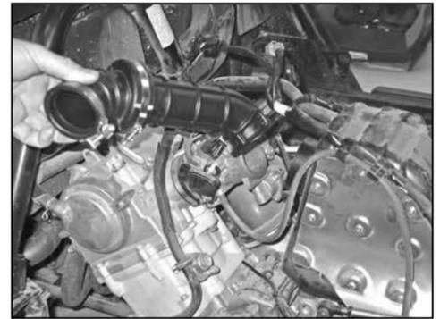
6. Remove the stock intake hose from throttle body and out of the air chamber as shown.
