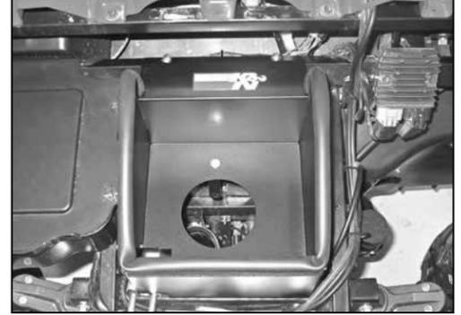
21. Install the heat shield assembly into the vehicle and secure with the provided hardware to the factory air box mounting locations.
