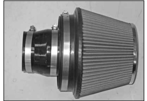
23. Install the silicone hose (08724) onto the filter adapter and secure with the provided hose clamp.
