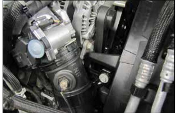
10. Reconnect the charge tube to the throttle body, be sure the locking ring has the charge tube locked onto the throttle body. Reinstall the charge tube mounting bolt.
