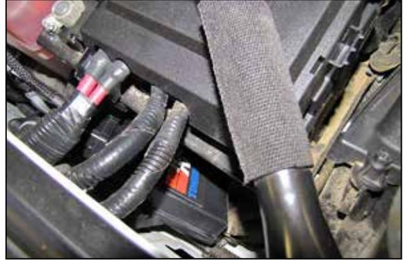
13. Secure the boost wiring harness to the boost module. Find a suitable location to secure the boost module and secure with the provided tie wraps.
