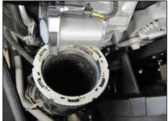
5. Release the charge pipe locking ring by rotating it clockwise and pulling the tube down away from the throttle body.
