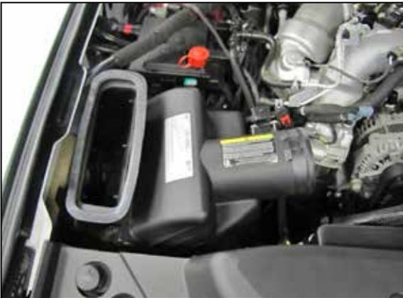
3. Lift the air filter housing assembly up and remove it from the vehicle.
