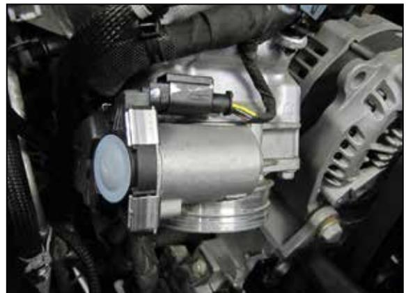
6. Disconnect the throttle body electrical connection and then remove the four bolts that secure the throttle body to the charge manifold. Remove the throttle body and gasket from the engine.
