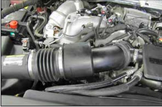
12. Reinstall the intake tube and secure with the factory hose clamps.
