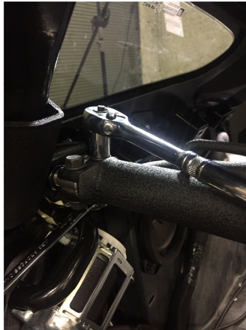
Step 15 Swap out provided install bolt for the factory seatbelt torx bolt (and attached belt assembly. Tighten. The provided install bolt is no longer needed and can be discarded.
