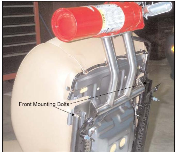
Figure 1.0 - Front Mounting Bolts
