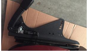
Step 3. Attach side mounts to aftermarket seats, using the hardware included with the seats. It is recommended that you fully tighten the inside (center console side) seat mount to mount bolts, but leave the outside seat mount somewhat loose until installed in the car. Seat height is set by the rear hole, seat tilt is set by the front holes.
