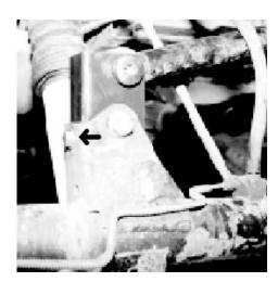
14. Check Brake Line Length, if they seem too short, longer stainless steel DOT Approved lines are available from Skyjacker. A driveline vibration may occur. If so, a transfer case lowering kit from Skyjacker should be installed.
