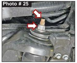
19mm wrench for nut & a 8mm wrench to hold shock stud. (See Photo # 25)
