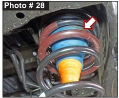
Note: Skyjacker Coil Spring Spacers Are Not Side Specific. Install Skyjacker Coil Spring Spacer into OEM rear coil spring mount with supplied 1/4" x 3/4" Bolt that is threaded into each Skyjacker spacer using a 7/16" wrench. (See Photo # 29)
