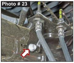
5. Disconnect OEM rear shock lower mount using a 17mm socket\wrench. (See Photo # 24) Tech Note: OEM shock perch runs at a downward angle. Lower\raise axle & compress shock to remove it.
