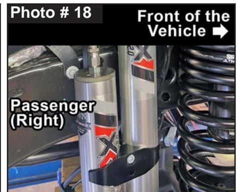
Connect Skyjacker shock at lower axle mount with OEM hardware using a 18mm socket \ wrench. Secure, but **Do Not Completely Tighten** at this time. These will be tightened once vehicle is on ground with full vehicle weight on tires \ wheels.
