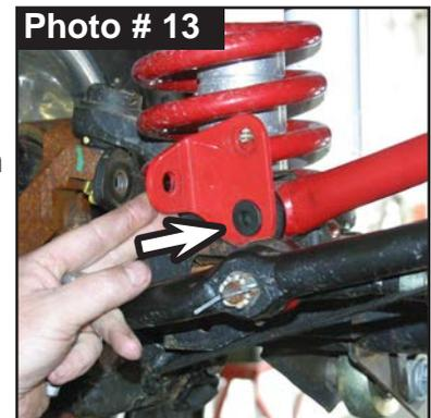
23. From # HB-TBA60 Hardware Bag, install Skyjacker Track Bar rod end by following the hardware pictured. (See Photos # 14 & # 15) Being sure to keep the rod end square (parallel) with the frame mount. On the rod end, rotate the jam nut against the steel tubing. Hold the rod end in place with a pipe wrench & use another pipe wrench or 1-1/8" wrench on the jam nut to completely tighten.
