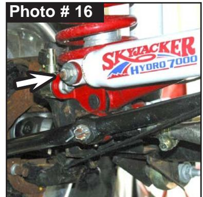
25. Apply a few drops of supplied # LT100 Thread Lock Compound onto the two (2) brake caliper OEM mounting bolts. Attach brake caliper to OEM knuckle using a 21mm socket \ wrench.
