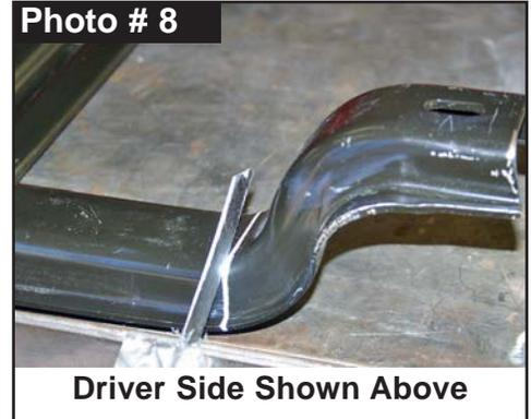
6. Using a reciprocating saw or similar tool, cut the outer mounting points off at the mark made in Step # 5. (See Photo # 8)
