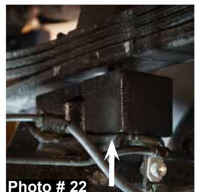
8. Disconnect the E-brake cable from the OEM leaf springs & install the new Skyjacker E-brake cable extension brackets to each OEM leaf spring using the OEM hardware, supplied 5/16" x 3/4" coarse thread bolts, washers, & nuts. (See Photo # 23)
