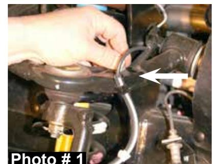
4. Remove the OEM ABS lines from the OEM upper A-arms & disconnect the OEM ABS / brake lines from the OEM steering knuckles. (See Photo # 1)
