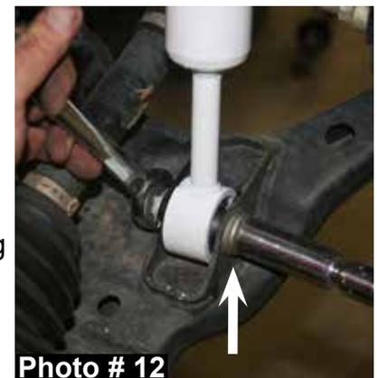
18. Connect the OEM upper strut mounts to the frame using the OEM hardware.
