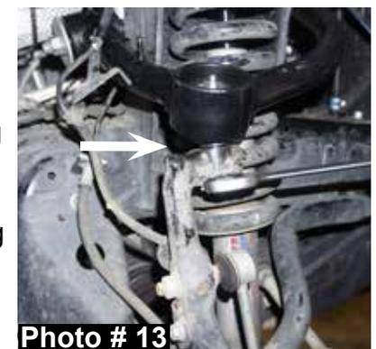
21. Connect the OEM outer tie rods to the OEM steering knuckles using the OEM hardware.
