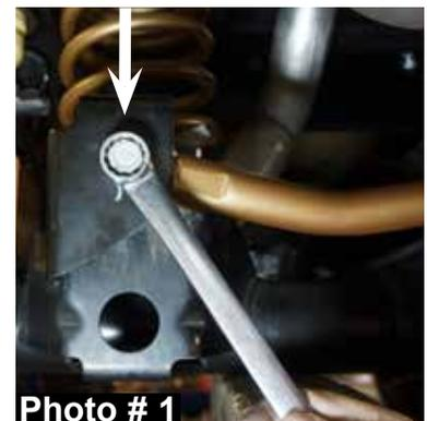
5. Using a tape measure, check the rear of the vehicle to make sure the body is centered over the rear tires / wheels & adjust the new Skyjacker rod end to align with the upper track bar mounting location.
