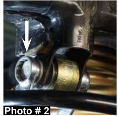
8. Tighten the supplied jam nut of the new Skyjacker adjustable rear track bar using a 1 1/8" wrench.
