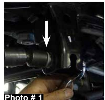
5. Using a tape measure, check the front of the vehicle to make sure the body is centered over the front tires / wheels & adjust the new Skyjacker rod end to align with the lower track bar mounting location.
