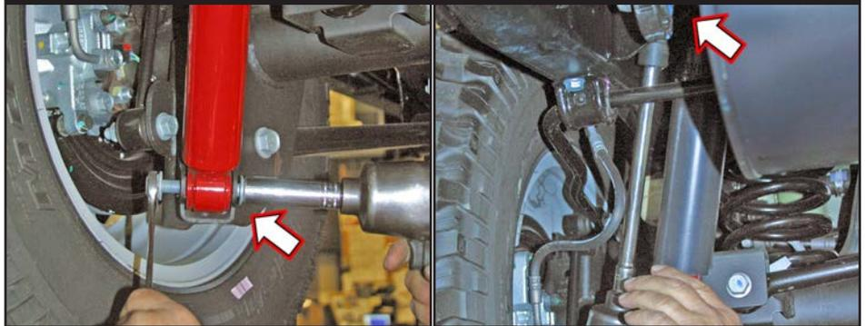
4. Disconnect OEM rear sway bar end link at axle mount using a 18mm socket \ wrench. (See Photo # 14)
