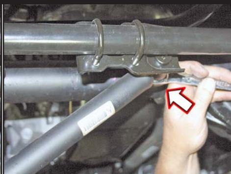
6. **Note:** If installing a Skyjacker OEM Replacement Steering Stabilizer, remove OEM steering stabilizer using a 18mm socket \ wrench. (See Photo # 3)
