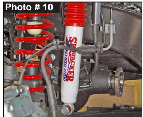
Connect Skyjacker shock at lower axle mount with OEM hardware using a 18mm socket \ wrench. Secure, but **Do Not Completely Tighten** at this time. To set bushings properly for ride height, these will be tightened once vehicle is on ground with full vehicle weight on tires \ wheels.
