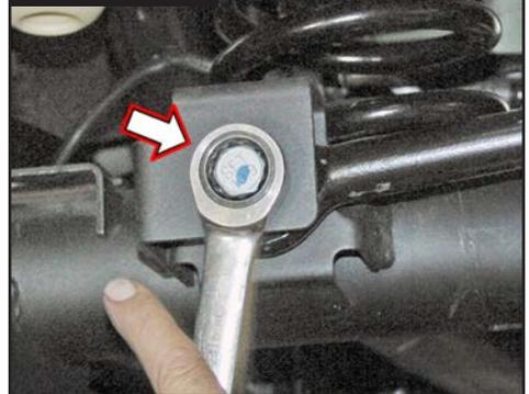
7. Lower the rear differential. Remove OEM rear coil spring & upper coil spring isolator.
