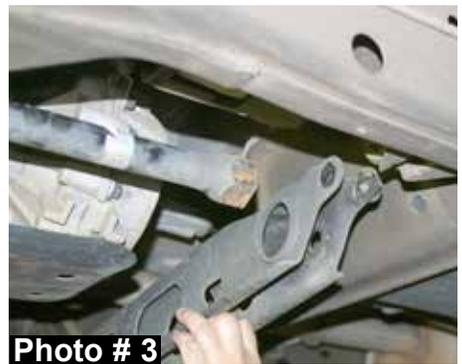
4. With the torsion bars removed from the rear cross member, remove the torsion bar cross member using a 21mm socket. With the cross member removed, remove the torsion bars from the vehicle. **Note:** Be sure to mark the torsion bars driver & passenger side for reinstallation. (See Photo # 3)
