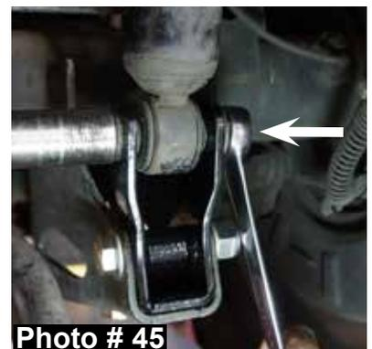
55. Air Ride models must also replace the OEM sensor link removed in step # 46 with the longer supplied link.
