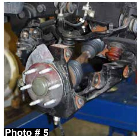
8. Remove the outer cv axle nut dust cover to allow access to the outer cv axle nut. Remove the outer cv axle nut & washer using a 1 7/16" socket. (See Photo # 6)
