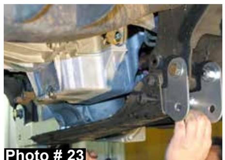
26. Install the new Skyjacker front cross member using the 5/8" x 4 1/2" fine thread bolts, washers, & nuts. **Note:** Be sure to install the anti-crush sleeves. (See Arrow in Photo # 24). If installing a new Skyjacker dual stabilizer, see those instruction sheets at this time.
