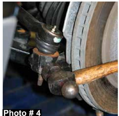
6. Remove the tie rod end nut from the steering knuckle using a 18mm socket. Remove the tie rod end from the steering knuckle by striking the knuckle to dislodge the tie rod end. **Note:** Be careful not to damage the tie rod end. (See Photo # 4)
