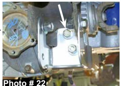
24. Place a washer on the 9/16" x 4 1/2" fine thread bolt. Install the bolt through the OEM rear differential mount, new cross member bracket, & frame.
