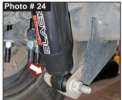
Install Skyjacker ADX rear shock. Connect upper shock mount with OEM hardware using a 21mm socket \ wrench. Connect lower shock mount with OEM hardware using a 21mm socket \ wrench. Secure, but **Do Not Completely Tighten** at this time.
