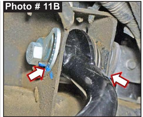
Secure, but **Do Not Completely Tighten** control arm hardware at this time. To set bushings properly for ride height, these will be tightened once vehicle is on ground with full vehicle weight on tires \ wheels.
