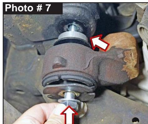
Tighten to All Four (4) Differential Mounts. Torque 120 ft-lbs. Remove jack from differential.
