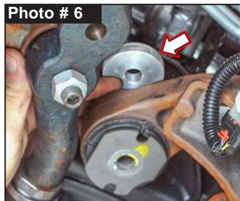
7. Remove two (2) rear OEM differential mount bolts using a 21mm socket \ wrench top & bottom.
