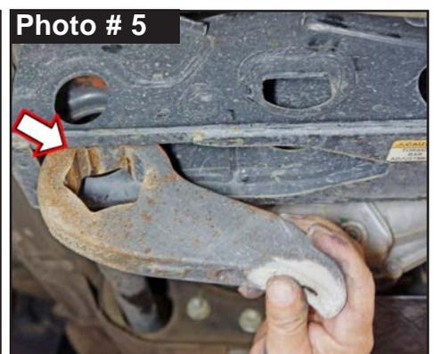
6. Place a jack or jack stand under front OEM differential to support weight of differential. Remove two (2) front OEM differential mount bolts using a 21mm socket \ wrench top & bottom.
