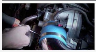
Loosen the clamps on the air intake tube and air box, and then remove the tube.
