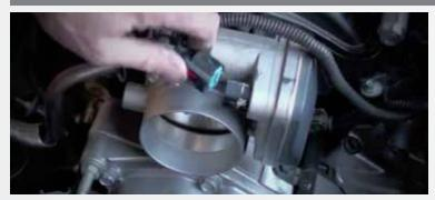
Remove the stock throttle body. The stock O-ring seal will be re-used. Be sure to wipe off and debris from the gasket.
