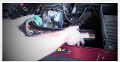
Re-install the air inlet tube to the BBK Throttle Body and air box and then tighten the clamps.
