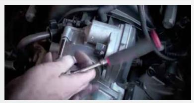
Bolt on the BBK Throttle Body using the stock hardware. On the 5.7L Hemi Plastic manifolds, take extra care when re-installing the mounting bolts. The "Speed Nut" type threaded nuts can be easily stripped. Make sure the threads of the bolts are properly engaged with the nut before tightening.
