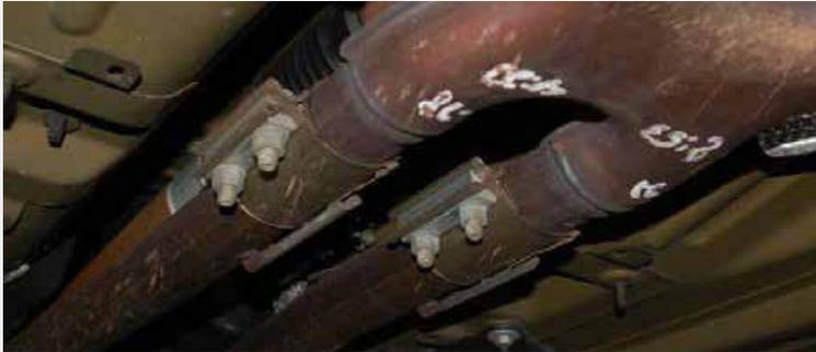
Separate the cat-back system by loosening the (2) 15mm nuts on each band clamp and prying the locking tabs up with a small flat head screwdriver while sliding the clamp towards the rear of the car.
