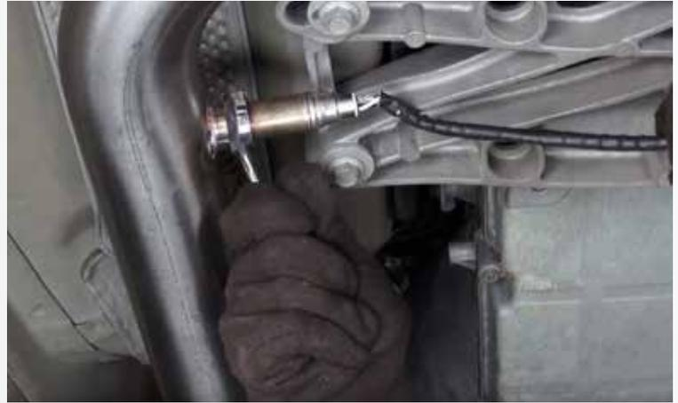
Remove the oxygen sensors from the stock pipes and install onto the BBK Mid-Pipes.
