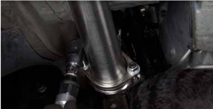
After installation of BBK Full Length Headers, install the matching Mid Pipes, rotate pipes as needed for alignment and fitment then start tighten at the collectors evenly and then the rear couplers ensuring the entire exhaust system is aligned correctly.
