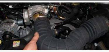
Disconnect the breather tube from the air intake tube. Loosen the clamps at the throttle body and at the air box then remove the air intake tube.
