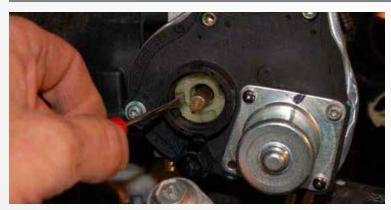
Using your small screwdriver, push in on the white spring retainer to release the spring. Unplug and remove the motor cover. Tighten the set screw for the brass adjuster stud. Reinstall the motor cover, reclock the internal spring counter-clockwise and lock the tabs into place. Reinstall the round plastic cover. Plug in the motor control wires.
