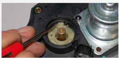
Pop off the round plastic cover on the motor cover. Install the cover on the throttle body. Using a small screwdriver, push the white spring retainer down while rotating it 160 degrees counter clockwise until the large and small tabs align with their slots. Release and allow the tabs to seat.
