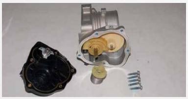
Remove the five Torq Head Screws and remove the motor cover and internal spring. Be aware that the cover will want to rotate as the screws are removed because of the internal spring being under some tension.
