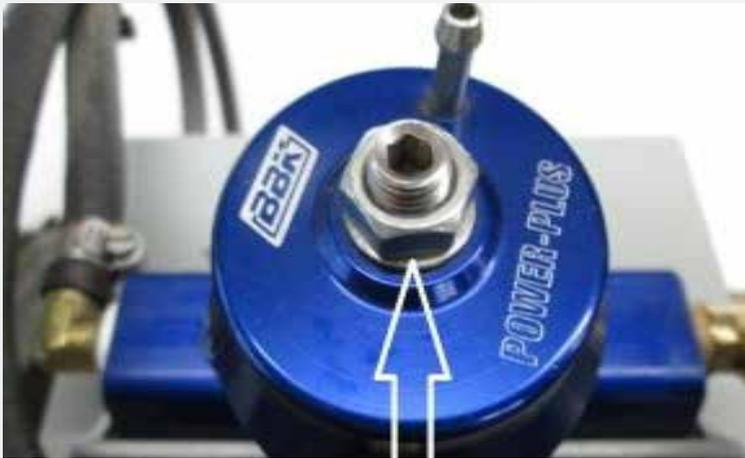
Loosen the lock-nut on the top of the fuel regulator.
