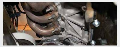
Place a jacking device under the bell housing and remove the driver side motor mount from the engine. This will give you access to the bottom row of header nuts.
