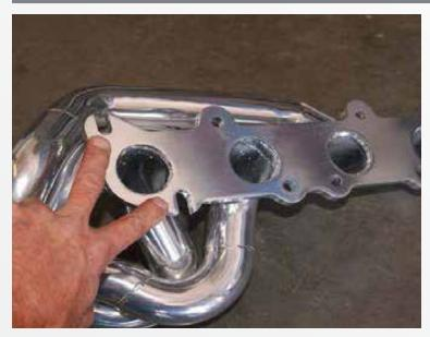
Looking at the BBK Header Flange, remove the studs that correspond with the notches in the flange. On the driver side it's the two most rear studs. Those will be replaced with supplied bolts.
