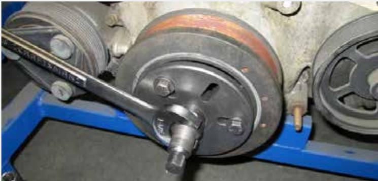
Remove the center bolt and washer from the factory pulley/dampener. Remove the alternator pulley and water pump pulley. Use a 3 prong harmonic dampener puller to remove the factory pulley/balancer. *cont. next column*
