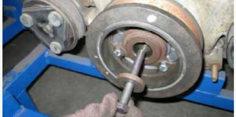
Attach the pulley assembly to the crankshaft using the new bolt provided and the original crank bolt washer. Use locktite or equivalent on the bolt and torque to 60 ft/lbs. Install the new water pump pulley using the original hardware. Also use locktite.
