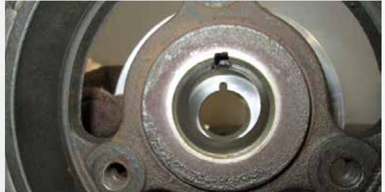
Install the hub of the factory harmonic balancer pulley into the counter bore of the BBK Pulley. Align the threaded hole in each pulley together. Install and hand tighten the (3) 1/4 x 1-1/4" bolts. The factory pulley does not completely sit into the under-drive at this point. Carefully tighten the (3) bolts equally in small increments to draw the (2) pulleys together. Remove the (3) 1/4" bolts.
