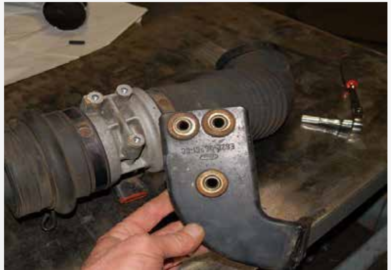
Remove the stock air box assembly.
