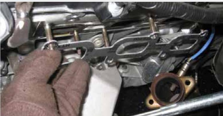
For both the driver side and passenger side place the supplied BBK Gasket and header into place. Then Tighten.
