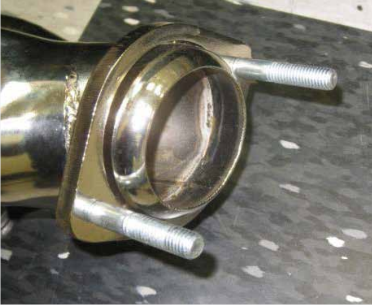
Install the supplied studs onto the BBK Header Collectors.
