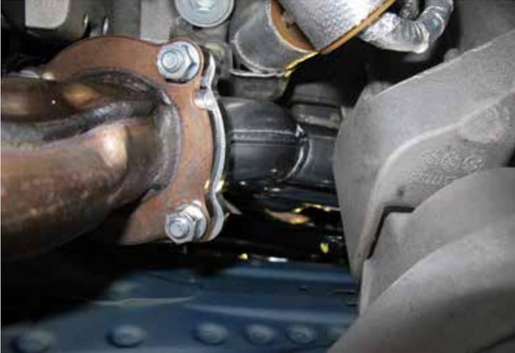
Install the supplied hardware to connect the catted mid pipe to the BBK tune length header and tighten it down, reinstall the steering shaft and tighten down its hardware.
