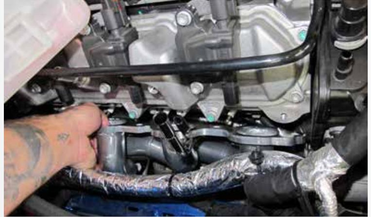
Install the BBK tune length header using the supplied gasket and hardware. **NOTE** the dipstick needs to be install at the same time by placing it through the header before putting it in.
