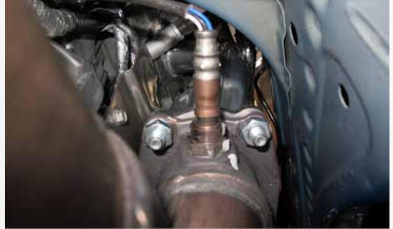
Install the (4) bolts supplied in the kit that connect the catted down pipe to the BBK tune length header and tighten them down.
