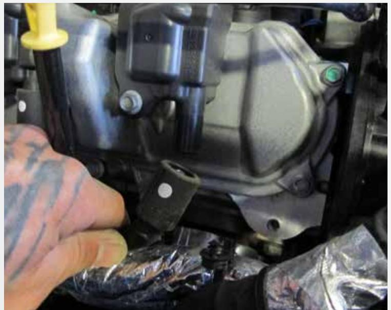
Remove the spark plug wires from the coil packs and the spark plugs.
