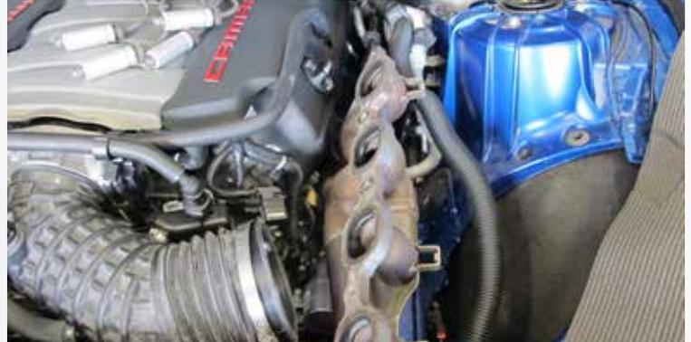
Remove the (5) bolts that secure the stock manifold to the cylinder head and remove the exhaust manifold and gasket from the vehicle.
