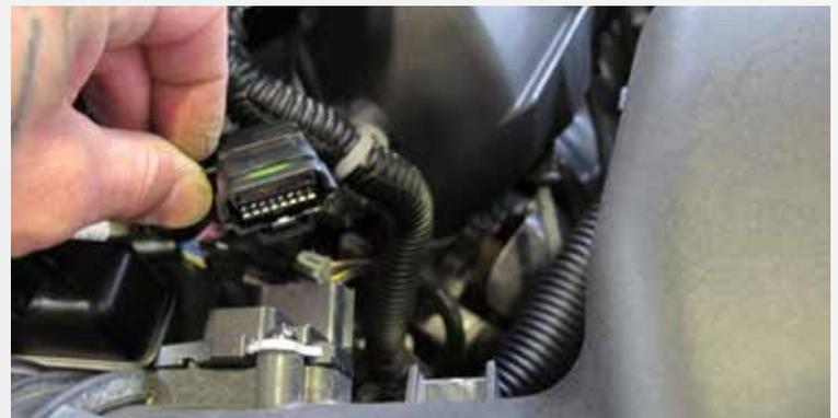
Unplug the wiring harness from the mass air sensor.
