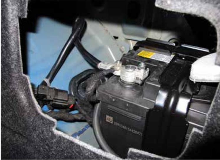
Disconnect the negative battery terminal located in the trunk of the vehicle.
