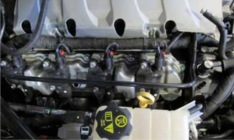
Reinstall the spark plug wires, dip stick hold down bolt, wiring harness bracket, reservoir bottle.
