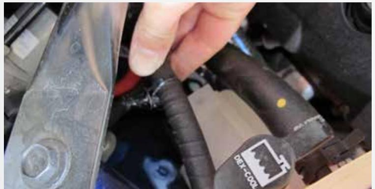
Disconnect the wiring harness from the reservoir bottle, remove the nut that secures the reservoir bottle to the chassis. Lift it up and it will lay up by the firewall.
