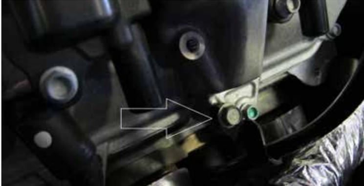
Remove the bolt that hold the oil dipstick in place.
