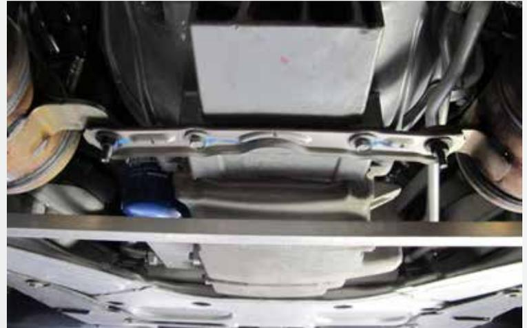
Tighten down the bolts on the cross brace. Reconnect the negative battery terminal after 500 miles of driving recheck and torque all hardware.
