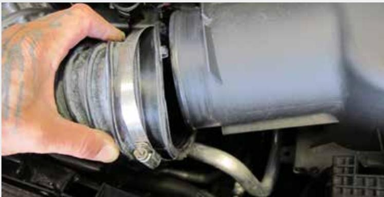
Loosen the clamp that secures the inlet tube to the factory air box, remove the air box by pulling it upwards releasing it from the rubber grommets and remove it from the vehicle.
