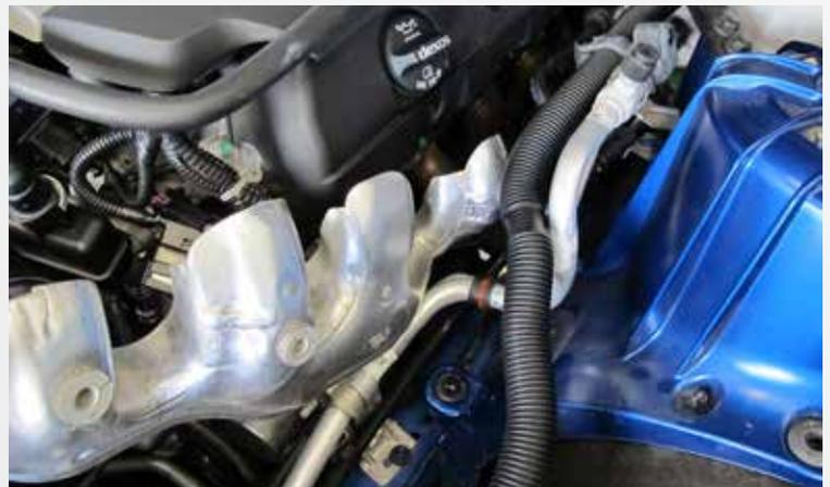
Passenger side remove the (3) bolts that hold the upper portion of the heat shield to the stock exhaust manifold and remove it from the vehicle.
