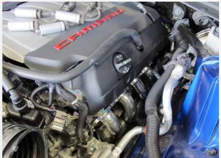
Install the BBK tune length header using the supplied gasket and hardware, tighten down the BBK tune length header bolts to the cylinder head first.
