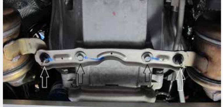
Loosen the (2) 13mm bolts and the (2) 13mm nuts on the cross brace. NOTE you do not need to remove it completely.
