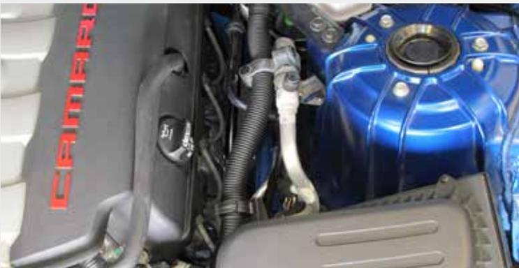
Reinstall the spark plug wires and the air box reconnect the mass air wiring harness and tighten down the clamp that connects the inlet tube to the air box.
