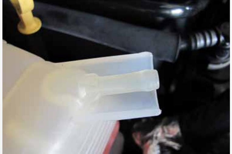
Driver side disconnect the upper radiator reservoir line from the reservoir using a bolt plug the end of the hose, using a rubber cap plug the reservoir bung.
