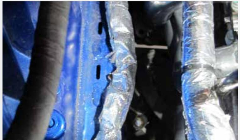
Tighten down all hardware on the header. Using the heat wrap supplied in the kit cover the lower wiring harness that runs along the body to protect it from any heat from the engine.
