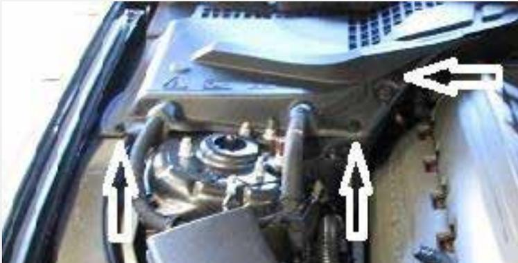
Remove the (3) pin screws that hold the battery cover to the chassis. Disconnect the negative battery terminal.
