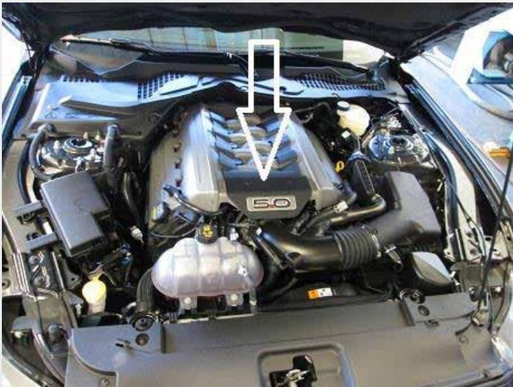
Remove the engine cover by pulling up on it to release its mounting pins from the grommets on the intake manifold.
