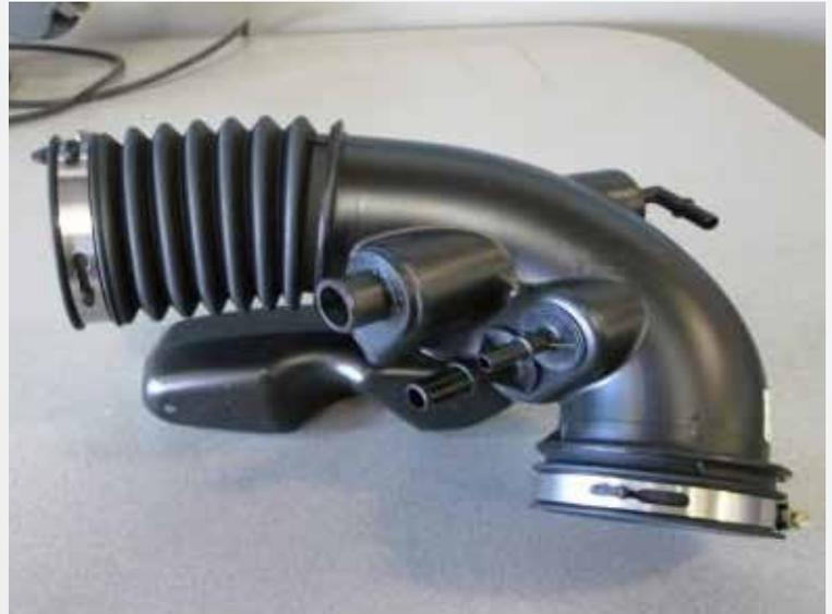
Loosen the (2) clamps on the air inlet tube at the air box and throttle body. And remove the air tube from the vehicle.
