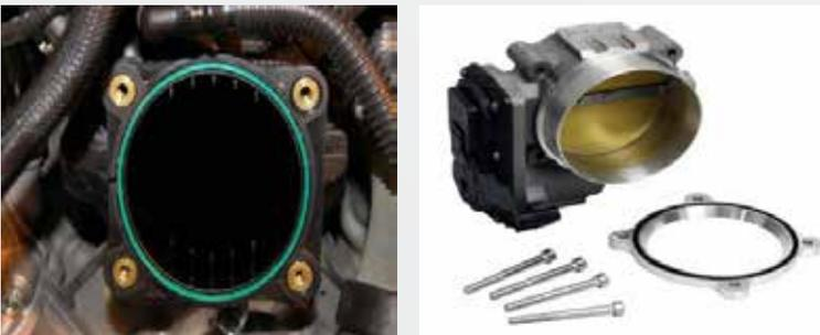
Wipe off the stock rubber throttle body gasket to remove any oil or debris. You will be reusing this gasket. Connect the motor plug to the BBK manifold. Use the supplied bolts to secure the throttle body to the intake manifold.
