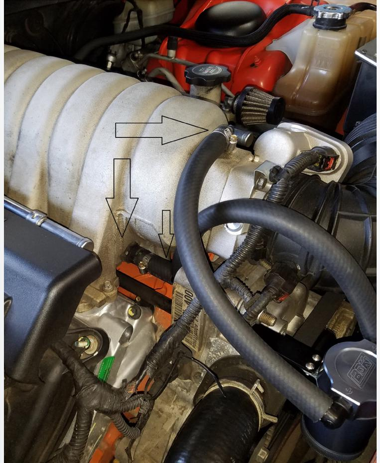
Install the vacuum hoses and clamps supplied in the kit. NOTE use the 90 degree fitting to connect the vacuum hose from the PVC to the BBK oil separator as shown in the picture.
