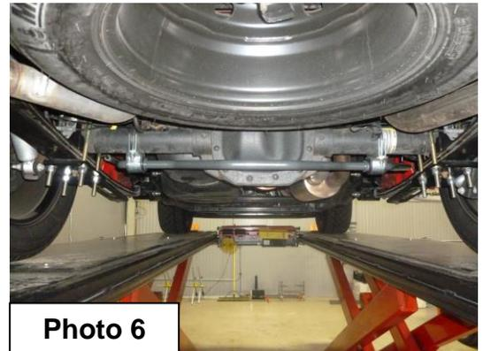
**WD-40™** is recommended to help remove excess lubricant. Re-greasing the pivot bushings should be Performed at regular intervals.
