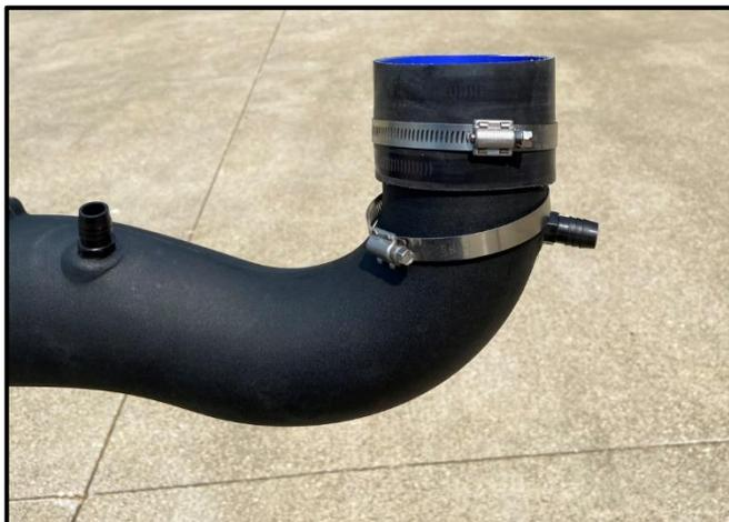
5. Locate the CORSA Air Intake Duct, the 2 Hose Clamps, the 2 Thread to Barb Fittings and either the Ø4in to Ø3.5in Reducer (6.2L) or Ø3.5in Hose (5.3L) (shown). Assemble the parts to the Air Intake Duct as shown. The Thread to Barb Fittings should be tightened until they are tight and flush to the mating surface on the Air Intake Duct. The hose clamps should be loose at this time.
