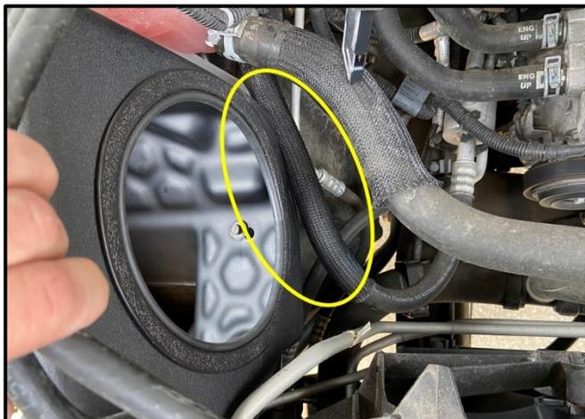
4. Before tightening the mounting bolts, ensure the hose shown in the oval is not under the Air Intake Box. This will hold the Air Intake Box up and not in place.
