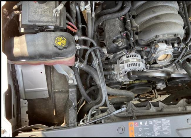
12. Remove the Factory Air Box Tray from the Vehicle.
