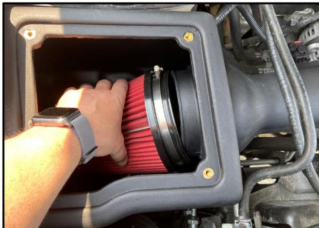
10. Next, locate the Filter (DryTech 3D shown). Insert the Filter into the Air Intake Box with the open side up. Turn the smaller end toward the fender, and then slide the open end onto the Air Intake Duct. Rotate the Filter or Clamp so the bolt on the Filter Clamp is accessible and use an 8mm Socket & Ratchet or Wrench to secure the Filter Clamp.
