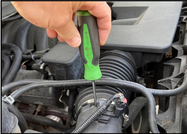
3. Using a T15 Torx Driver, remove the Factory MAF Screws. These will not be reused. Next, disconnect the Mass Air Flow (MAF) Sensor from the Wire Harness by pulling the red clip up and then squeeze the sides of the Wire Connector to release it. Carefully remove the MAF Sensor and store it in a safe location. It will be reused in Installation Step 9.
