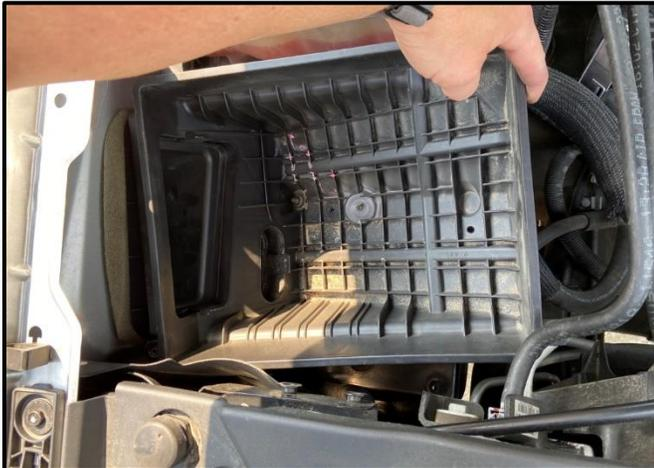
10. Lift the Factory Air Box Lid from the Factory Air Box Base. To remove the Base, lift the right side up to release it from the Grommets, and then pull the Base toward the engine to release the base from the Fender. This will not be reused.
