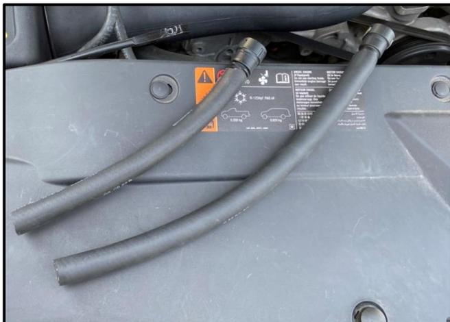
7. Locate the 2 Hoses and 2 Quick Connect Fittings. Press the fittings into one end of the hoses, as shown.
