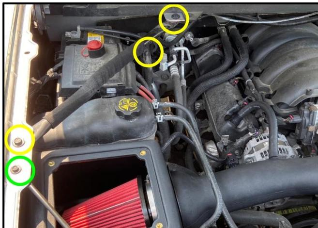
11. Locate the Fender Brace and 3 Bolts from Removal Step 1. Using a 14mm Socket & Ratchet or Wrench, reattach the 3 bolts and the Fender Support into the vehicle in the circled in **YELLOW** areas. Torque them to factory specs.
