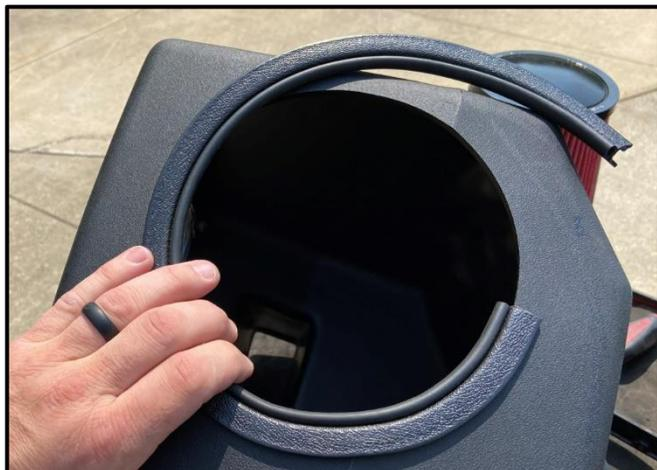
1. Locate the CORSA Air Intake Box and the Box Opening Seal. Starting on the bottom of the opening, press the Seal around the opening.
