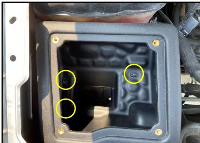
3. Align the Mounting Slots in the bottom of the Air Intake Box to the Factory Mounts. Then, locate the bolts for the Factory Air Box Mounting Tray in Removal Step 11. Hand thread 3 of the Bolts into the Factory Mounts. Make sure the Air Intake Box is close as you can get it to the Fender.
