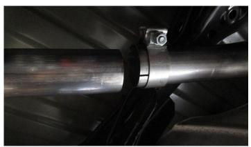
9. Install a 2.5" clamp into the inlet of the driver's side rear tailpipe and insert the driver's side rear tailpipe into the driver's side front tailpipe. Place the driver's side rear tailpipe hanger into the factory grommet as shown in **Step 10.** Secure the clamp. Do not fully tighten at this time.
