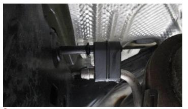
Place the front muffler hanger in the factory grommet.
