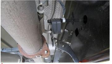
Remove hanger from the front of the muffler using grommet puller, or a similar device.
