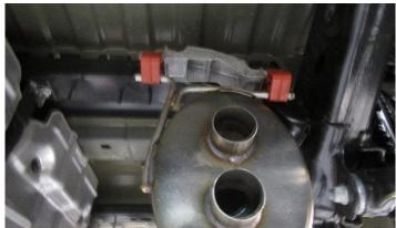
3. Install the rear muffler hangers in the factory grommet assembly. (5.7L Muffler shown)
