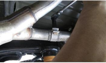
2. Loosen the passenger side tailpipe clamp using a 15mm deep socket or wrench.
