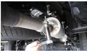
**3.** Loosen both of the tip clamps and remove the factory tip assemblies using a 13mm deep socket or wrench.
