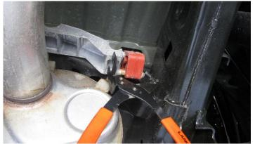
**5.** Remove both of the hangers from grommets at the back of the muffler using a grommet puller or similar device.
