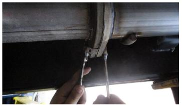
Using a 17mm socket or wrench and a 15mm socket or wrench, secure the flange connection with the supplied hardware.
