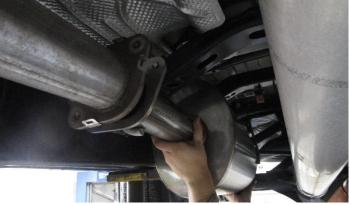
Line up muffler as shown in the picture. Align the flange to the mating flange of the mid pipe. (5.7L Muffler Shown)
