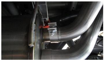
Install a 2.5" clamp into the inlet of the driver's side front tailpipe then insert the driver's side front tailpipe on the top outlet of the muffler. Secure the clamp using a 15mm socket or wrench. Do not fully tighten at this time.
