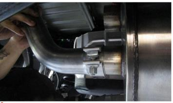
Install a 2.5" clamp into the inlet of the passenger side front tailpipe as shown, then insert the passenger side tailpipe on the bottom outlet of the muffler. Secure the clamp using a 15mm socket or wrench. Do not fully tighten at this time.
