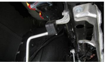
**10.** Placing the hangers on the driver, and passenger side rear tailpipe.
