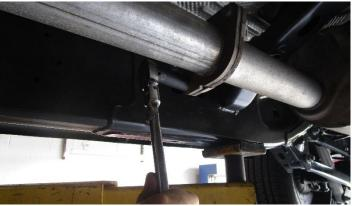
Loosen and remove the two muffler flange bolts that secure the muffler inlet flange using a 16mm socket or wrench.
