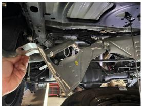
B. The spare tire and the driver side heat shield will need to be lowered in order to provide clearance for the removal of the remaining stock exhaust as noted in the next step. Using a 10mm socket unbolt the two bolts from the frame rail and only loosen the third bolt at the passenger heat shield connection.
