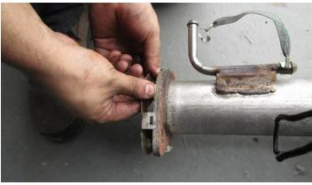
**9.** Carefully guide the rest of the system towards the front of the vehicle and down to remove the system completely from the vehicle.
