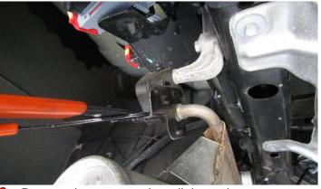
Remove hangers on the tailpipe using a grommet puller, or similar device.
