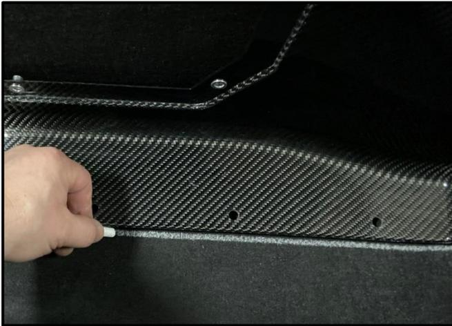
3. Using a piece of Chalk or a similar NON-permanent method of marking, draw an outline around the entire CORSA Carbon Fiber Trunk Panel onto the Trunk Carpet.
