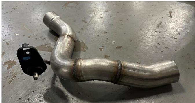
5. Locate the passenger side axle pipe assembly, and the hanger grommet assembly removed during **REMOVAL STEP 7** of the stock exhaust removal process. Install the hanger grommet assembly onto the front hanger of the muffler assembly in the same position as previously installed on the stock exhaust.
