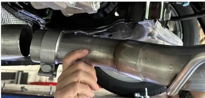
7. Slide the axle pipe inlet pipe over the passenger side X-pipe outlet. **NOTE:** The use of a soap and water solution may aid in the installation of hanger grommets.
