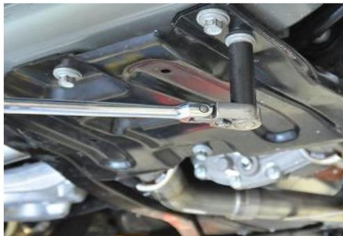
1. Loosen the furthest front bolt holding the driver side factory convertible brace using a 3/8" drive ratchet and 13mm deep socket. Loosen the bolt so there is about a 1/4" – 1/2" gap between the bolt head and the brace. Do not remove the bolt completely. Remove the factory driver side convertible brace by removing the remaining 7 bolts, working your way from front to rear; then slightly lowering the brace and sliding it rear wards.
