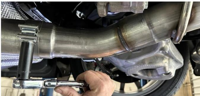
9. Tighten the clamp connecting the passenger axle pipe to the passenger side X-pipe outlet using the 3/8" ratchet and 15mm deep socket until the axle pipe assembly is snug on the X-pipe.
