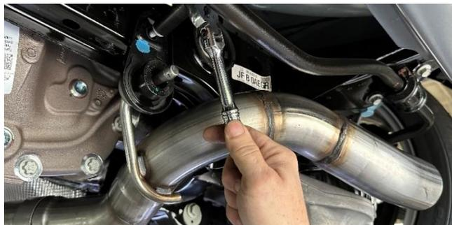
8. Locate a 13mm bolt set aside during **REMOVAL STEP 5** of the stock exhaust removal process. Install the front passenger hanger grommet assembly onto the rear suspension sub-frame and tighten it down with the 13mm bolt, 3/8" ratchet and 13mm socket.
