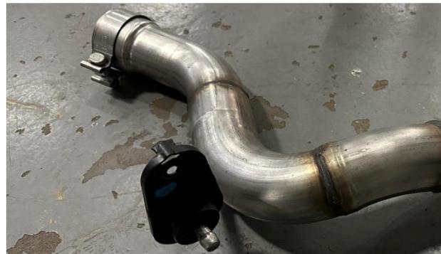
6. Locate one 3" clamp. Install the clamp on the passenger side muffler inlet pipe so that the bolt is vertical with the nut towards the ground and the bolt is towards the inside of the vehicle.
