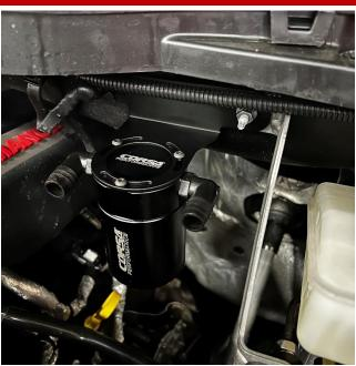
Locate the bolt and nut on the driver's side firewall that holds the coolant reservoir. Remove the nut using a 10mm socket and install catch can and secure it by reinstalling the nut.
