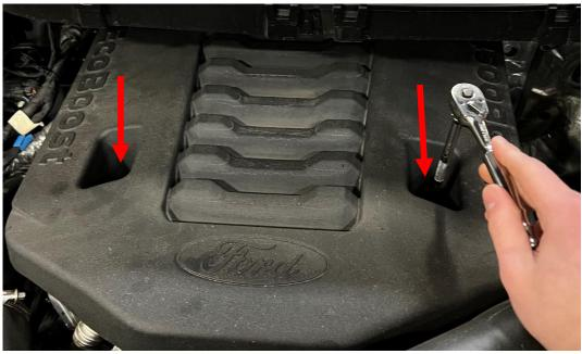
1. Remove the 2 nuts from the bolt that hold down engine cover using a 10mm socket wrench. Pull engine cover out towards the front of the vehicle.
