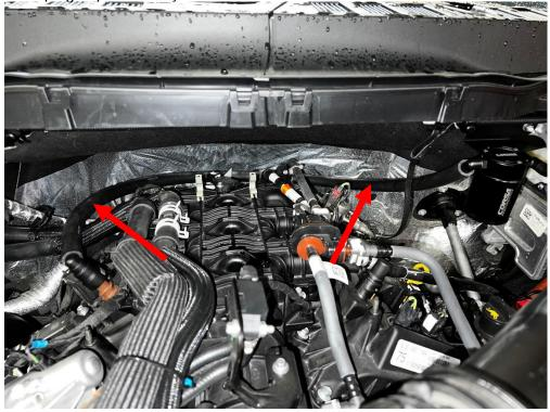
3. Install quick disconnect fittings to one end of each hose. Attach hose A to the A end of the catch can and route the hose along the firewall to connect it to the BROWN fitting on the engine.
