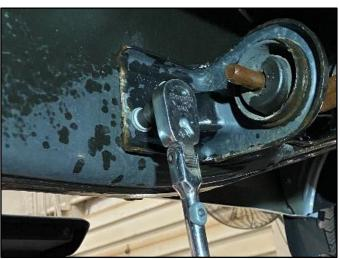
Using a 10mm socket & ratchet, remove the 2 bolts securing the front hanger mount to the chassis. Set aside the 2 Bolts in a safe place. They will be reused during INSTALL STEP 11.
