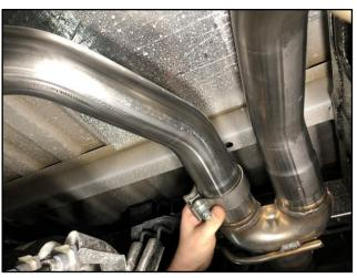
18. Repeat INSTALL STEPS 14-17 to install the CORSA driver split pipe and CORSA driver tailpipe. Note that both driver hangers are located on the driver tailpipe.
