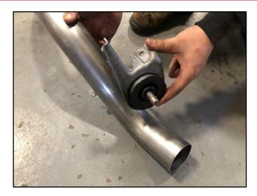
5. Locate the CORSA passenger split pipe assembly. Install the front tailpipe hanger mount as shown onto the hanger location of the CORSA split pipe. Make sure to orient the hanger mount in the same way as on the factory exhaust system.
