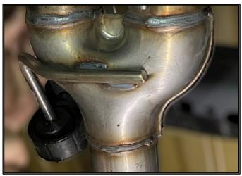
3. Install the mid hanger mount as shown onto the rear hanger location of the CORSA mid pipe. Make sure to orient the hanger mount in the same way as on the factory exhaust system.
