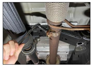
Using a 15mm socket & ratchet, loosen the factory clamp securing the factory muffler section to the factory head pipe.
