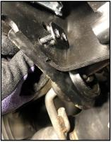
4. Using a 10mm socket & ratchet, remove the 2 nuts securing the passenger rear tailpipe hanger mount and mounting bracket to the chassis. Remove the mounting bracket to free the rear tailpipe hanger mount from the vehicle. Set aside the 2 nuts and the mounting bracket in a safe place. They will be reused during INSTALL STEP 17.
