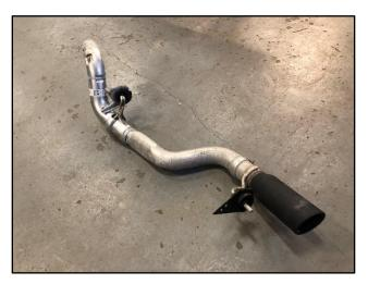
**5.** Carefully remove the passenger side factory tailpipe from the vehicle.
