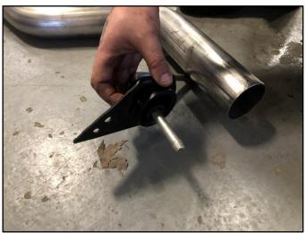
**6.** Locate the CORSA passenger tailpipe assembly. Install the rear tailpipe hanger mount as shown onto the hanger location of the CORSA tailpipe. Make sure to orient the hanger mount in the same way as on the factory exhaust system.
