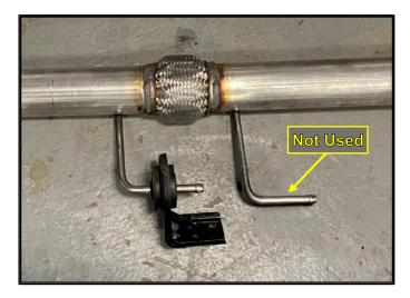
Locate the CORSA mid pipe, then Install the front hanger mount as shown onto the forward hanger location.
