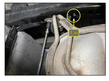
**9.** Locate the mid hanger mount above the back of the factory rear muffler. Using a 10mm socket & ratchet with a long extension, remove the bolt securing the hanger mount to the chassis. Next, pull the hanger mount towards the center of the vehicle and then downwards to release the hanger mount locating tab from the chassis. Set aside the bolt in a safe place. It will be reused during INSTALL STEP 12.
