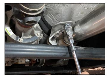
**9.** Locate the head pipe flange bolts from **REMOVAL STEP 11**.
