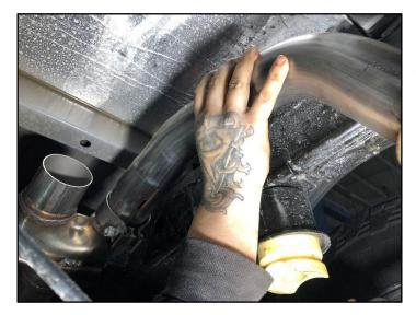
14. Locate the CORSA passenger split pipe and one of the 2.75in clamps from the hardware kit. Position the clamp onto the inlet of the CORSA split pipe.
