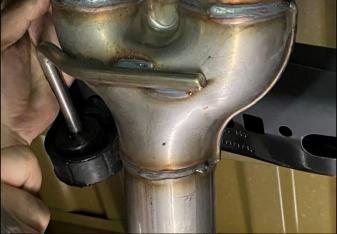
12. Locate the bolt for the mid hanger mount from REMOVAL STEP 9. While supporting the CORSA mid pipe, insert the tab on the hanger mount into the hole in the chassis and carefully thread the bolt through the hanger mount and into the factory clip nut in the chassis. Use a 10mm socket & ratchet with a long extension to SNUG the bolt.
