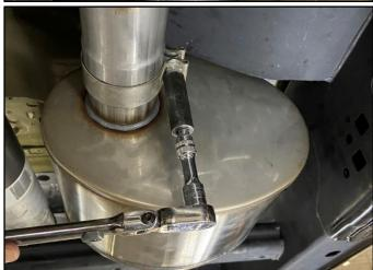
13. Confirm the pipe joint overlap and clearances to the vehicle, and make sure the outlet of the CORSA mid pipe is level with the ground, then use a 15mm socket & ratchet to SNUG the clamp connecting the CORSA mid pipe to the CORSA muffler.
