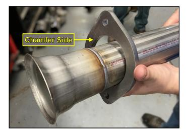
**8.** Locate the CORSA head pipe and the head pipe flange from the hardware kit. Assemble the head pipe flange onto the head pipe, with the chamfer side facing towards the flare.
