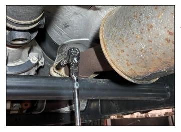
11. Using a 13mm socket & ratchet with extension, loosen the two bolts securing the stock flange connection on the factory head pipe. A second person may be needed to support the head pipe when the two bolts are loosened.
