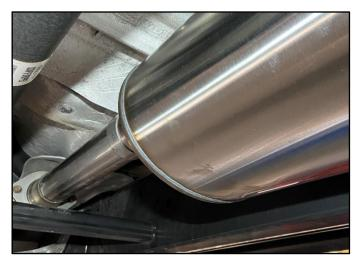
Locate the CORSA muffler and one of the 3in clamps from the hardware kit. Position the clamp onto the inlet of the CORSA muffler.
