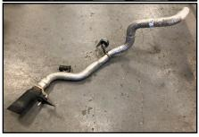
**6.** Repeat **REMOVAL STEPS 1-5** to remove the driver side factory tailpipe from the vehicle.
