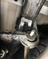
3. Using a 10mm socket & ratchet, remove the 2 bolts securing the passenger front tailpipe hanger mount to the chassis. Set aside the 2 Bolts in a safe place. They will be reused during INSTALL STEP 15.
