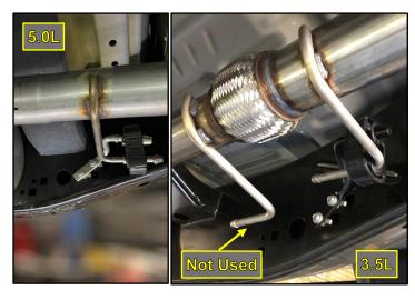
Locate the CORSA mid pipe and one of the 3in clamps from the hardware kit. Position the clamp onto the inlet of the CORSA mid pipe.
