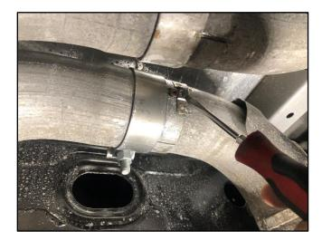
Identify the passenger side factory tailpipe connection located above the rear differential on the passenger side of the vehicle. Using a Small flat head screwdriver, pry open the locking tab to free the tailpipe locating key from the factory muffler section.
