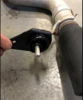
With the factory passenger tailpipe section on the ground, use grommet pullers or similar device to remove the two tailpipe hangers from the corresponding hanger mounts. Note the orientation of the hanger mounts before removal for the next two steps.
