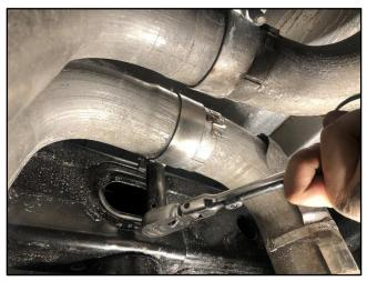
Using a 15mm socket & ratchet, loosen the factory clamp securing the passenger side tailpipe to the factory muffler section.
