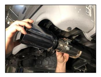
19. Locate one of the CORSA tip assemblies and one of the 2.75in clamps from the hardware kit. Position the clamp onto the inlet of the CORSA tip assembly.
