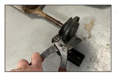
With the factory muffler section on the ground, use grommet pullers or similar device to remove the two factory muffler hangers from the corresponding hanger mounts. Note the orientation of the hanger mounts before removal for the next two steps.
