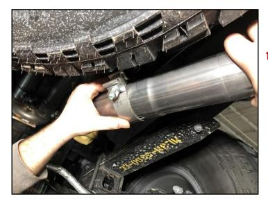
**16.** Locate the CORSA passenger tailpipe and one of the 2.75in clamps from the hardware kit. Position the clamp onto the inlet of the CORSA tailpipe.
