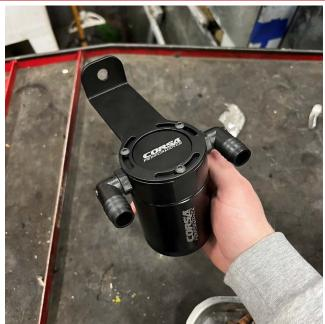
Locate your vehicle's PCV line and remove it. Find a mounting location for your Corsa Catch Can. Use the provided bracket(s), fittings, and hose to route the catch can to the PCV system. The A end of the catch can is the inlet, the B end of the catch can is the outlet. **IMPORTANT:** Corsa Performance highly recommends applying PTFE tape or thread sealant to the fittings and the bottom drain plug to avoid any leaks.
