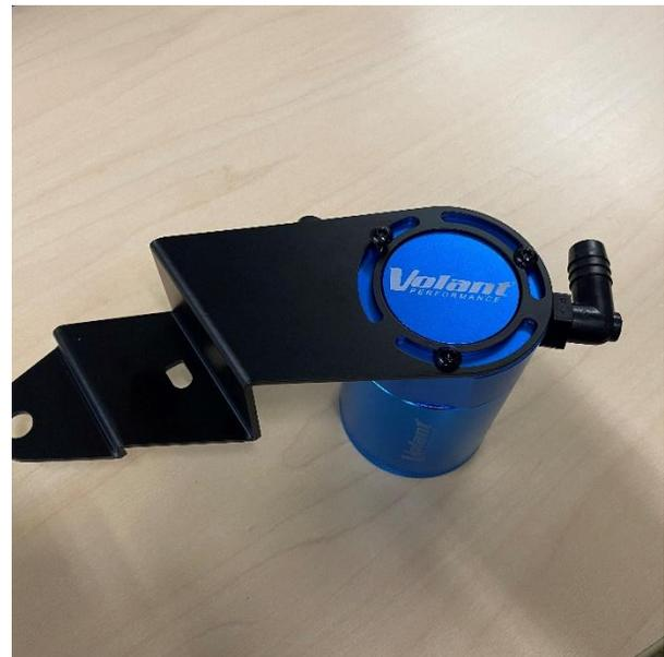
1. Install both 90 degree barb to 3/8" NPT fittings to the catch can using an 11/16" wrench. The barbed end of the fitting should be facing away from the vertical Volant logo on the catch can body. **IMPORTANT:** Volant highly recommends using thread sealant or PTFE tape on threaded fittings to prevent any leaks.
