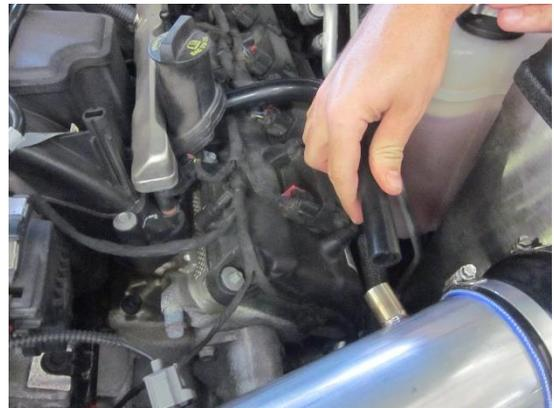
14. Install supplied breather hose onto Volant duct and factory location on engine.
