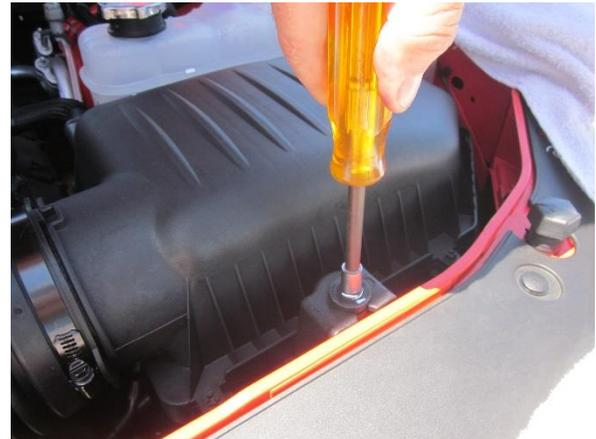
6. Remove bolt securing factory air box to vehicle using 8mm socket and ratchet.
