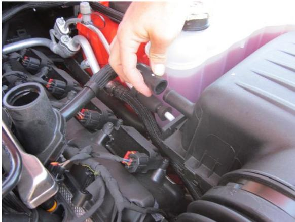
5. Disconnect vacuum hose from factory air box and engine.
