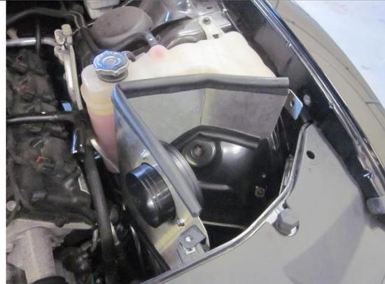
6. Place Volant shield assembly into vehicle.
