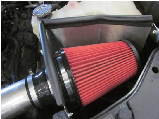
13. Place filter on adapter and tighten clamp using 8mm socket and ratchet.
