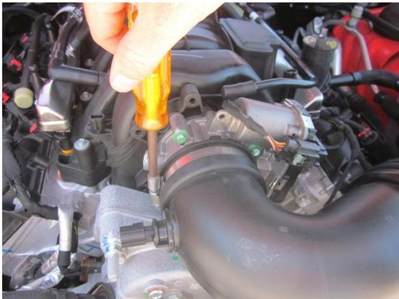
3. Loosen clamp securing factory air duct to throttle body using 5/16" socket and ratchet.
