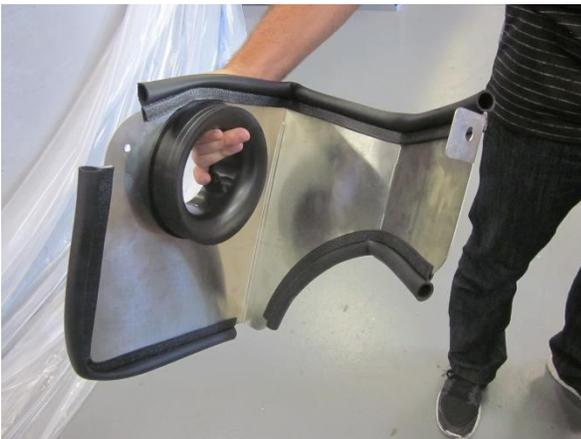
3. Install vinyl trim pieces to Volant shield. Add relief cuts at sharp bends to ease installation.
