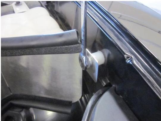
7. Place spacer between shield and inner fender and insert 6mm x 30 bolt with 1/4" lock washer and 1/4" flat washer. Tighten bolt with 10mm socket and ratchet.
