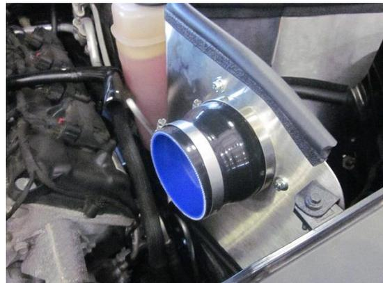
10. Install reducer onto filter adapter along with #64 clamp placed loosely on large end and #60 clamp placed loosely on small end.
