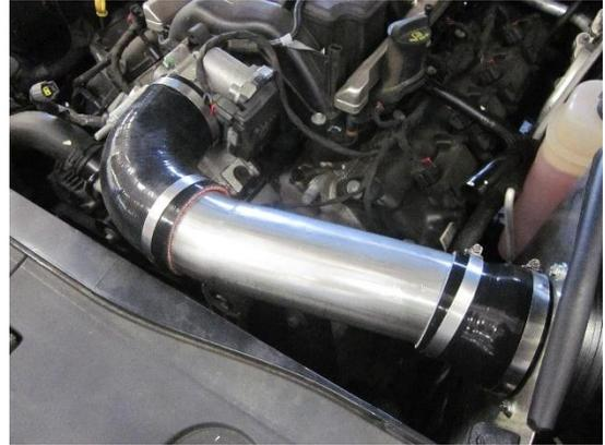
12. Push Volant duct into hump hose and onto throttle body. Adjust duct as necessary and tighten all four clamps using an 8mm socket and ratchet.
