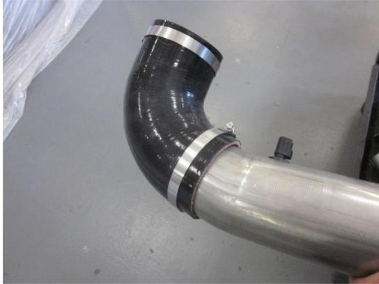
11. Place straight sleeve onto end of Volant duct along with two #60 clamps placed loosely.
