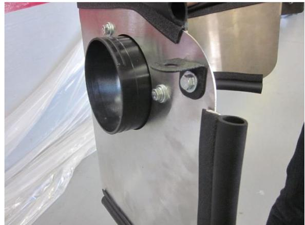
4. Loosely assembly bracket to shield using 6mm x 16 bolt, 1/4" lock washer, two 1/4" flat washers, and 6mm nut.
