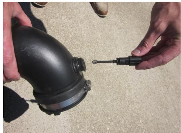
8. Remove ATS from factory air duct.
