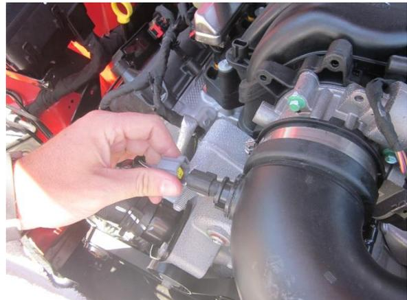
4. Disconnect wiring harness from air temperature sensor (ATS).
