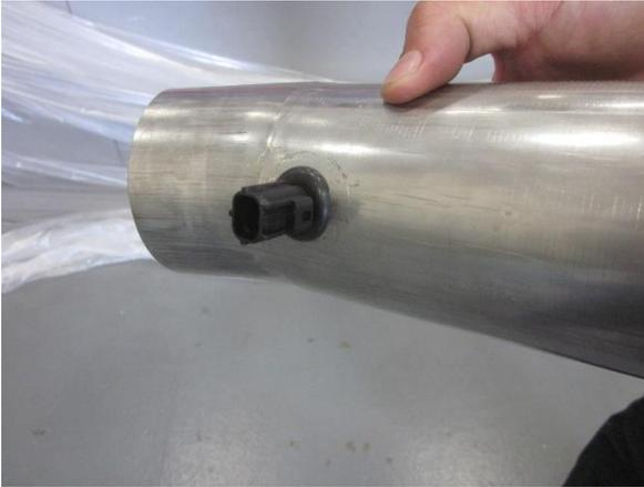
1. Install supplied rubber grommet into Volant air duct. Install factory ATS from removal step 8 into grommet.
