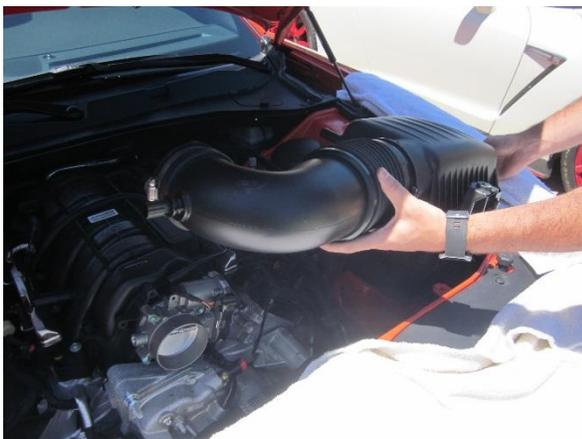
7. Pull factory air duct off throttle body and lift entire factory intake up and out of vehicle.
