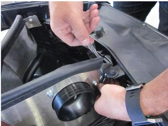
9. Tighten shield hardware from step 4 using two 10mm wrenches.
