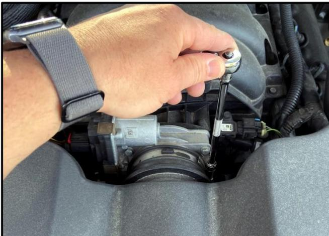
5. Using an 8mm Socket & Ratchet or Wrench, loosen the Hose Clamp connecting the Factory Air Duct to the Throttle Body. This will not be reused.
