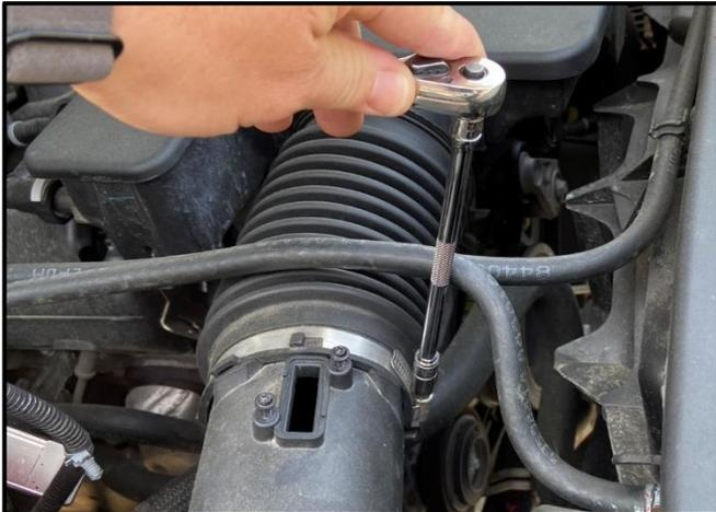
4. Using an 8mm Socket & Ratchet or Wrench, loosen the Hose Clamp connecting the Factory Air Duct to the Factory Air Box. This will not be reused.
