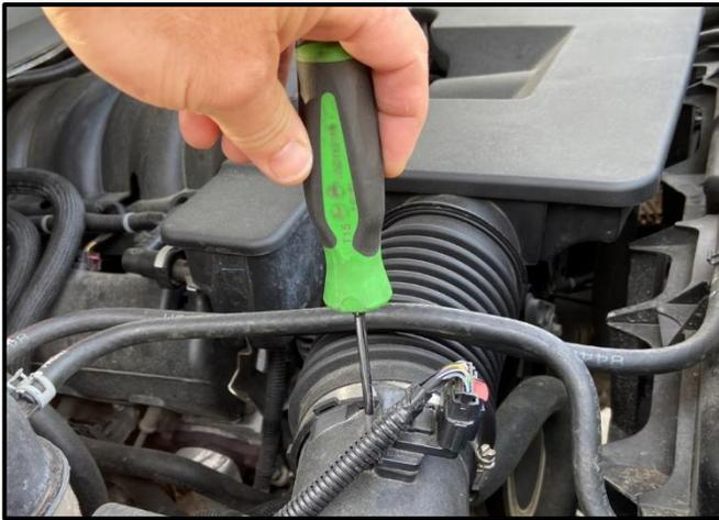
3. Using a T15 Torx Driver, remove the Factory MAF Screws. These will not be reused. Next, disconnect the Mass Air Flow (MAF) Sensor from the Wire Harness by pulling the red clip up and then squeeze the sides of the Wire Connector to release it. Carefully remove the MAF Sensor and store it in a safe location. It will be reused in Installation Step 9.
