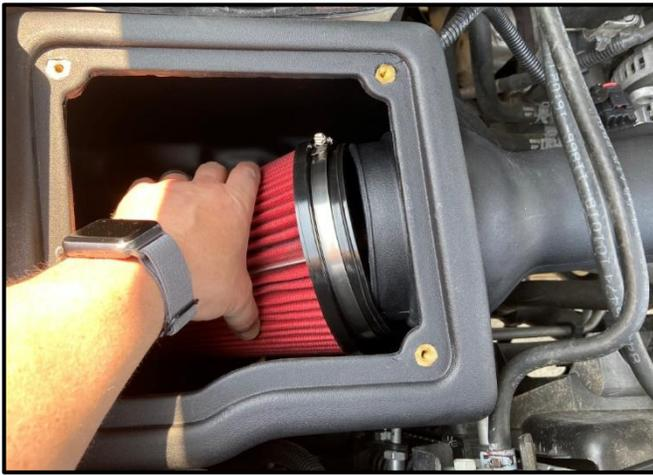
10. Next, locate the Filter (DryTech 3D shown). Insert the Filter into the Air Intake Box with the open side up. Turn the smaller end toward the fender, and then slide the open end onto the Air Intake Duct. Rotate the Filter or Clamp so the bolt on the Filter Clamp is accessible and use an 8mm Socket & Ratchet or Wrench to secure the Filter Clamp.
