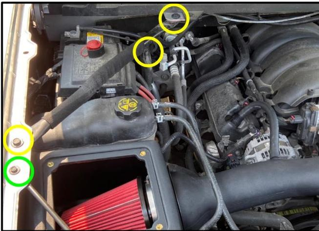
11. Locate the Fender Brace and 3 Bolts from Removal Step 1. Using a 14mm Socket & Ratchet or Wrench, reattach the 3 bolts and the Fender Support into the vehicle in the circled in **YELLOW** areas. Torque them to factory specs.
