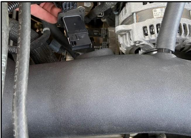
9. Locate the MAF Sensor Gasket and install it onto the MAF Sensor removed in from Removal Step 3. Next, slide the MAF Sensor and Gasket into the opening in the back of the Air Intake Duct. The Flat Side goes up and the screws will only align one way. Then locate MAF Screws from the Hardware Kit and use a Phillips Screwdriver to secure the MAF Sensor to the Air Intake Duct. Once the MAF Sensor is secured, reconnect the Wire Harness and push the Red Locking tab down.
