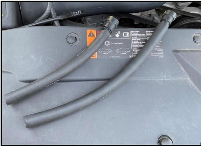
7. Locate the 2 Hoses and 2 Quick Connect Fittings. Press the fittings into one end of the hoses, as shown.
