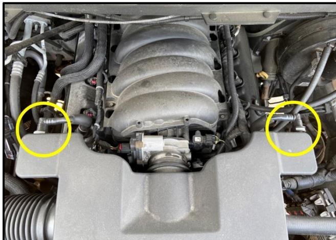
6. Locate the Factory Quick Connections on the rear of the Factory Air Duct. Squeeze the Grey Tabs and pull the Connections off the Factory Duct and rotate the Stock Hoses out of the way.
