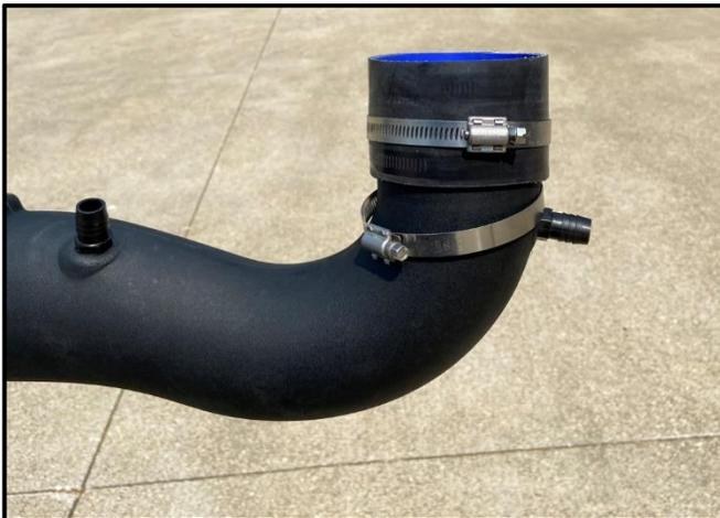
5. Locate the Volant Air Intake Duct, the 2 Hose Clamps, the 2 Thread to Barb Fittings and either the Ø4in to Ø3.5in Reducer (6.2L) or Ø3.5in Hose (5.3L) (shown). Assemble the parts to the Air Intake Duct as shown. The Thread to Barb Fittings should be tightened until they are tight and flush to the mating surface on the Air Intake Duct. The hose clamps should be loose at this time.
