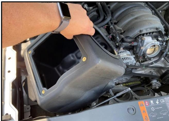
2. After the Seal is installed, install the Air Intake Box into the vehicle. This is done by sliding the Side Inlet Duct through the opening in the Fender and the Lower Inlet Scoop through the opening above the fender.
