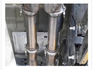
**Step 10:** Once an xMod option has been chosen, loosely attach the assembly to the flange ring outlet of the Inlet Assemblies using the supplied V-Band clamps.
