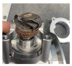
**Supplemental step 1**: The valves are supplied assembled, it is necessary to remove the top plate to perform the next step. Remove the Clocking Spring (heatsink) from the OE assembly and install it onto the Magnaflow valve as shown.
