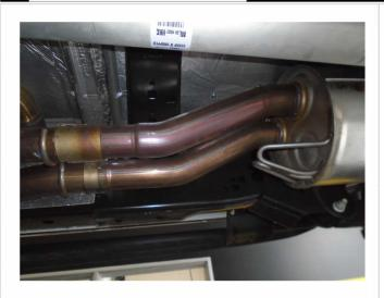
**Step 3:** Begin removal of your OE system by first loosening the clamps in front of the muffler assembly and un-plugging the electrical connections to the valves. Disengage all welded hangers from the rubber insulators. Retain the large slide clamp(s) and rubber insulators as they will be used to install your new system.
