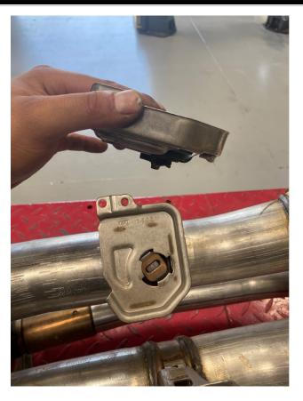
**Step 6:** Begin by removing the valve motor assembly from the OE exhaust. At this point you will need to plug the motor assembly back into the wire loom on the vehicle to reset the motor location, this is done by opening/closing the driver side door. Remove the Motor assembly, it is now ready to be installed onto the MagnaFlow valve.
