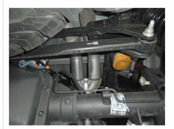
**Step 4:** Next loosen the clamps on both pipes where they pass over the rear axle. With the exhaust supported working front to back remove the OE exhaust system. You will also need to remove the spare tire to install this system. You are now ready to install your new MAGNAFLOW exhaust system
