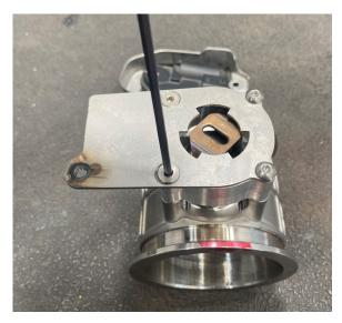
**Supplemental step 2**: Once the Clocking Spring is installed reassemble the valve in the order it was disassembled. Take note that the machined spacers have two countersunk holes and they must correspond with the countersunk holes in the plate and the flat head machine screws.
