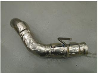
**Step 8:** Before beginning the exhaust installation the heatshield from the OE system needs to be moved to the MagnaFlow system. Cut the retaining straps securing the heatshield. Move it over the MagnaFlow Over Axle Assembly and secure using the supplied 3.00" worm drive clamps.
