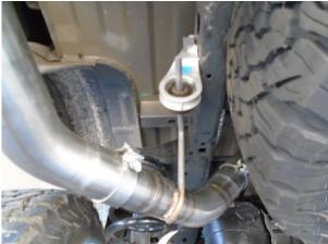
**Step 14:** Attach the D/S extension Pipe and the Mid-Pipe Assemblies to the X-Pipe using the supplied clamps and fitting the hangers into rubber insulators.
