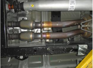
**Step 1:** This kit supplies Inlet pipes to replace the resonator pipes on the 5.2L(R) and can replace the equal length (Loop) pipe assembly on the 3.5L. These supplied pipes can be used for a more aggressive sound but aren't necessary to complete the installation. If using these pipes begin removal at Step 2. if not continue to Step 3.
