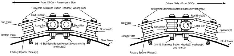
Check to make sure that you have all parts listed prior to installation. If anything is missing contact us immediately.
